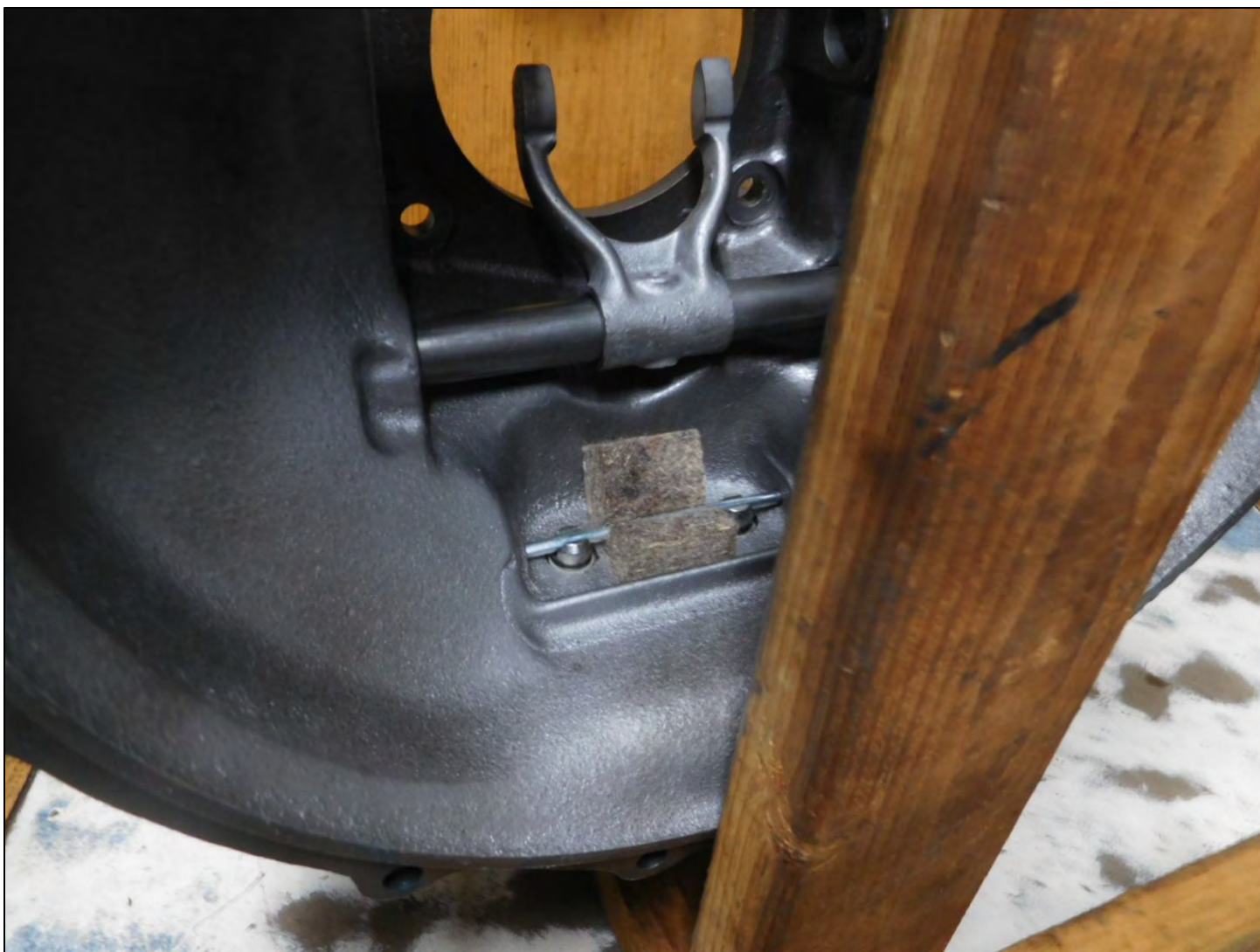
New front wishbone bolts, felt, and pin installed along with a new clutch release shaft and housing bushings.
