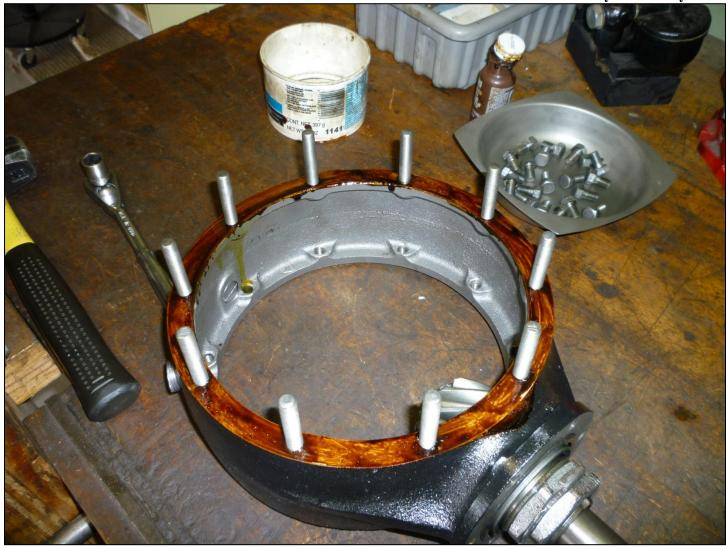
This is the final assembly of a differential overhaul. The photo shows the right side of the banjo with the gaskets coated with Indian Head gasket sealer. Both sides of all gaskets are coated. The threaded studs are used to align the gaskets with the bolt holes.
