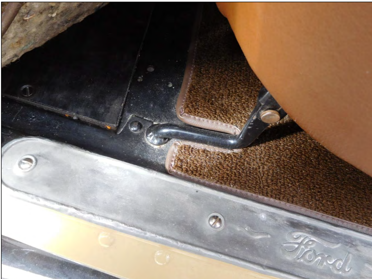
The extended pivot stud installed on the driver's seat of Ben's 1930 Tudor.
