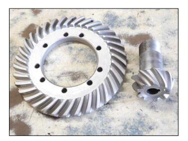
Shown in the photo above is an original 378:1 ring & pinion gear set. The dimensional lines can be seen on the pinion sleeve in the middle of the sleeve. The photo on the right shows the first bearing being pressed on with an interference press fit.
