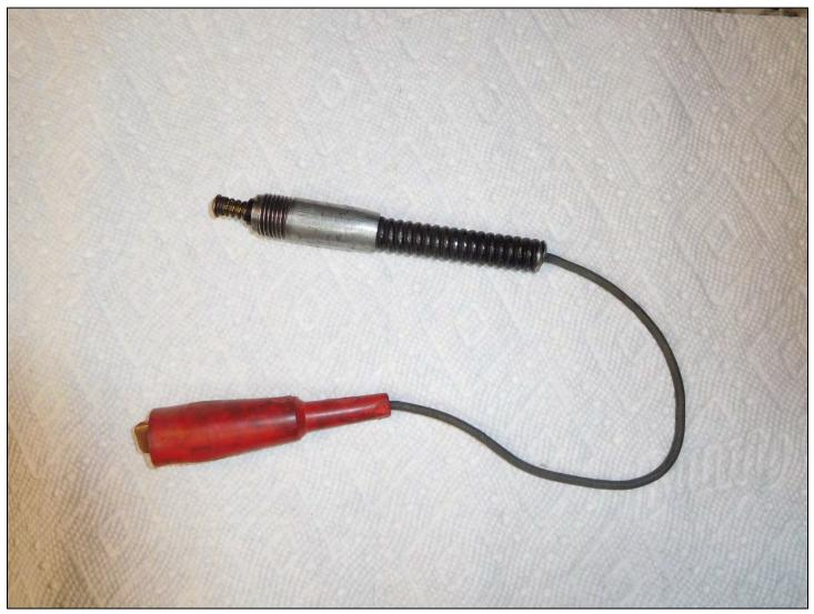
The threaded end of the bypass cable screws into the distributor, the clip end is attached to the coil where the red wire was removed. A bypass cable can be fabricated using the threaded end of a discarded pop-out cable. Some Model A suppliers also carry factory made versions. Bratton's Antique Auto offers them under part number 16360, \$18.35.
