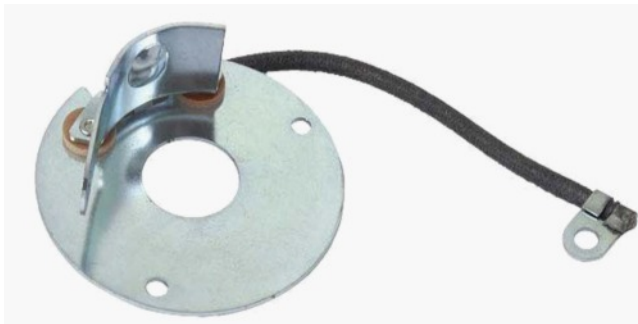
Lower plate with correct connecting wire
