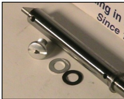
Distributor shaft with oil hole
