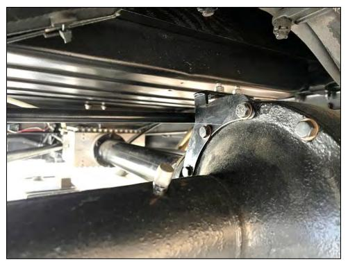
The vent is an Alemite 304810 air vent valve. 1" OAL 1/8" PTF. Overall length 1.0 inches, shank length 0.19 inches. Cost is about \$5.
