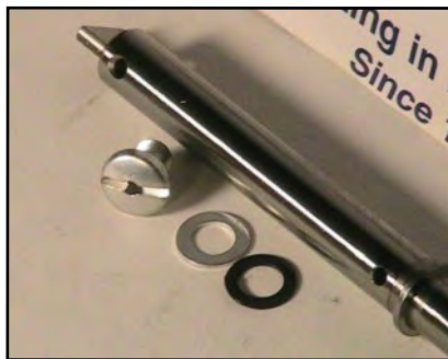
Distributor shaft with oil hole
