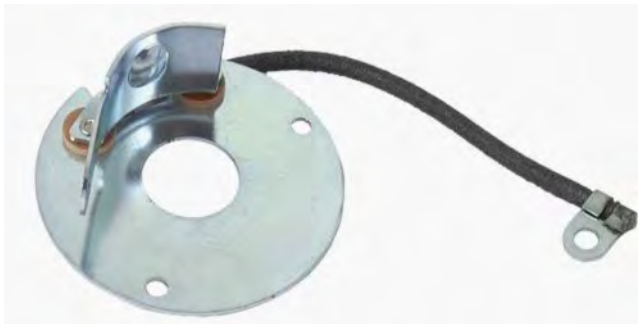
Lower plate with correct connecting wire
