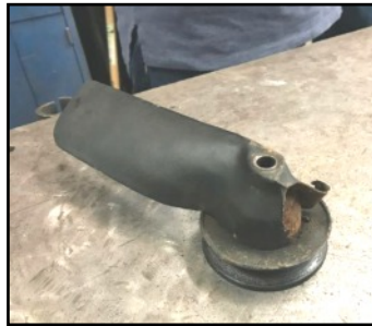
Original Model A fan that failed
