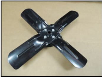
Poor quality replacement fans that use bolts to attach the blades to a steel or aluminum hub
