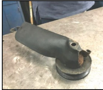
Original Model A fan that failed
