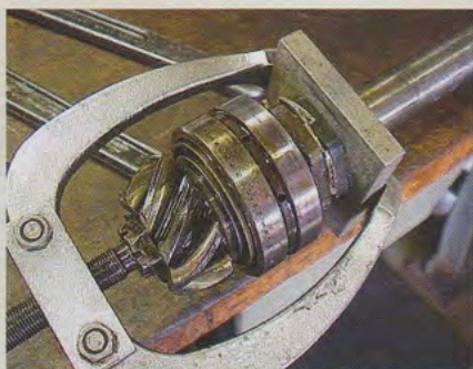
#15. A flywheel puller and a backing device are used to remove the pinion assembly from the drive shaft. Tighten the puller sufficiently and tap the end of the puller with a hammer. Continue tightening and tapping until the pinion breaks loose from the taper on the drive shaft.
