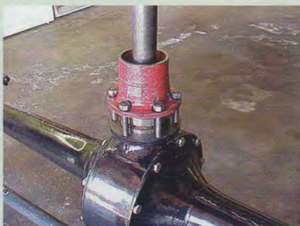
#18. The pinion gear assembly with the Mitchell stub shaft installed is re-inserted into the banjo using a tool made from a cut off torque tube. Tighten the six nuts evenly while rotating the stub shaft to engage the pinion gear with the ring gear. Continue tightening until the pinion assembly is fully seated.
