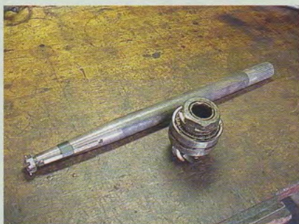
#17. The Mitchell stub shaft is inserted into the pinion in place of the drive shaft. Torque the 15/16" hex nut to a nominal 100 foot-pounds.
