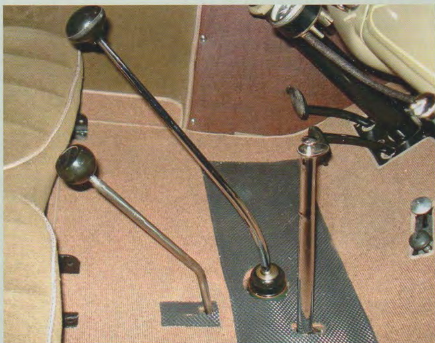
#23. The Mitchell shifter is located behind and to the right of the standard shifter. Shift it forward and you are in overdrive. Shift it backwards and you are out of overdrive. The overdrive can be used in any gear and is particularly beneficial in second gear-overdrive when driving in mountainous terrain.
