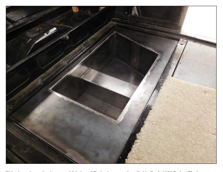
This photo shows the sheet metal fabricated Tudor basement installed in Ben's 1930 Tudor. The basement is sitting on the metal rails that the floorboard attach to. The floorboard was placed over it and the mounting screw holes were marked on the basement. With the holes drilled out in the basement, the mounting screws go down through both the floorboard and the basement. The basement was later painted black inside and out.
