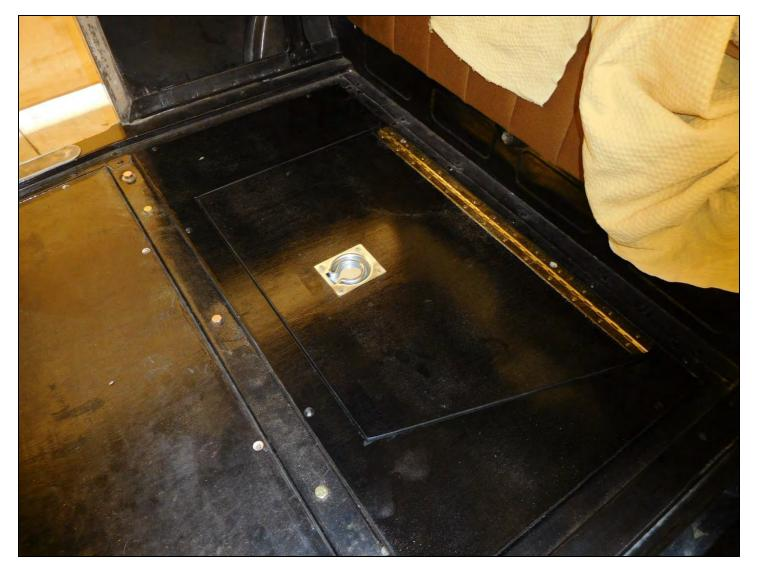
This photo shows the floorboard installed with the trap door cut into it. The piano hinge and the pull handle were procured from Home Depot.
