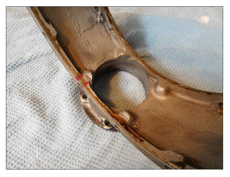
This photo show an additional crack in the banjo from the 1930 Tudor that is on the lip on the left side of the banjo flange where the left axle housing bolts on. There are also two witness marks on the left side where a ring and pinion bust-up must have occurred sometime in the past.
