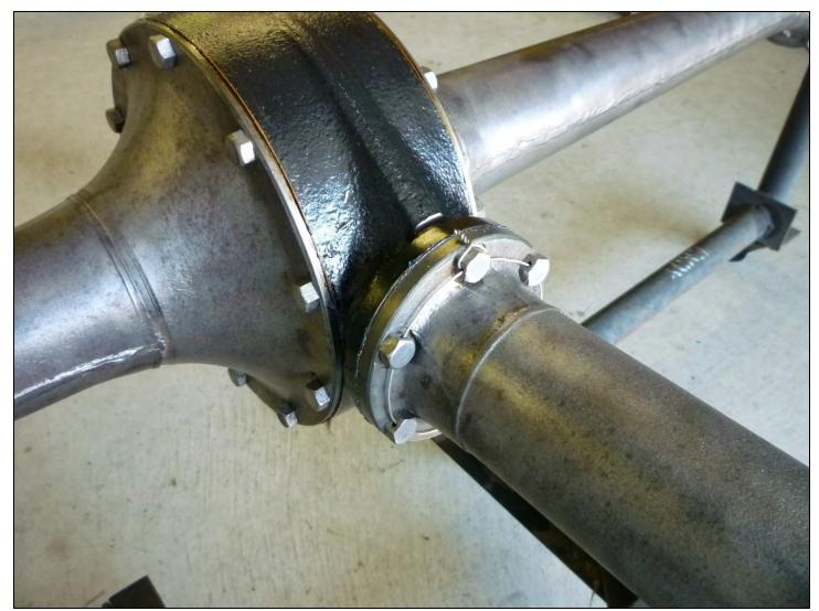
The top support gusset is seen directly above and to the left of where the safety wire terminates. There is an identical gusset on the bottom. The torque tube attaches to the banjo flange and is secured with six retaining bolts and is safety wired.
