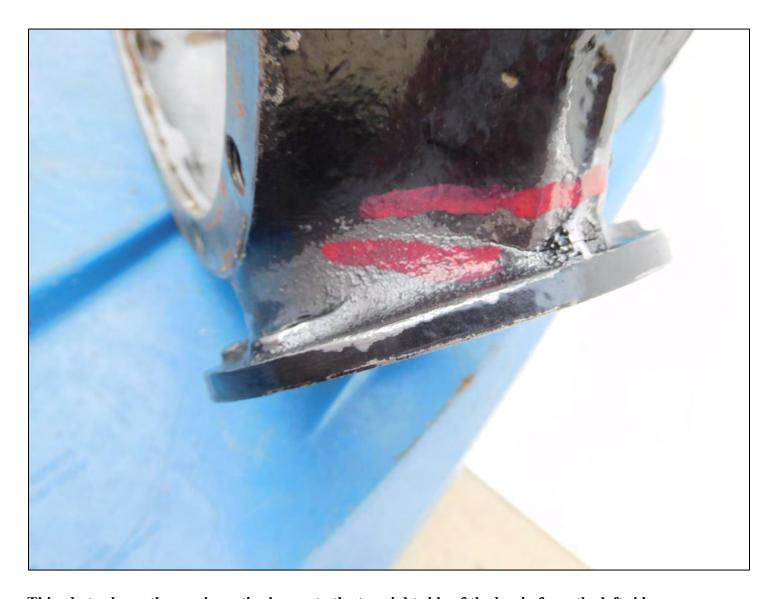
This photo shows the crack continuing on to the top right side of the banjo from the left side.
