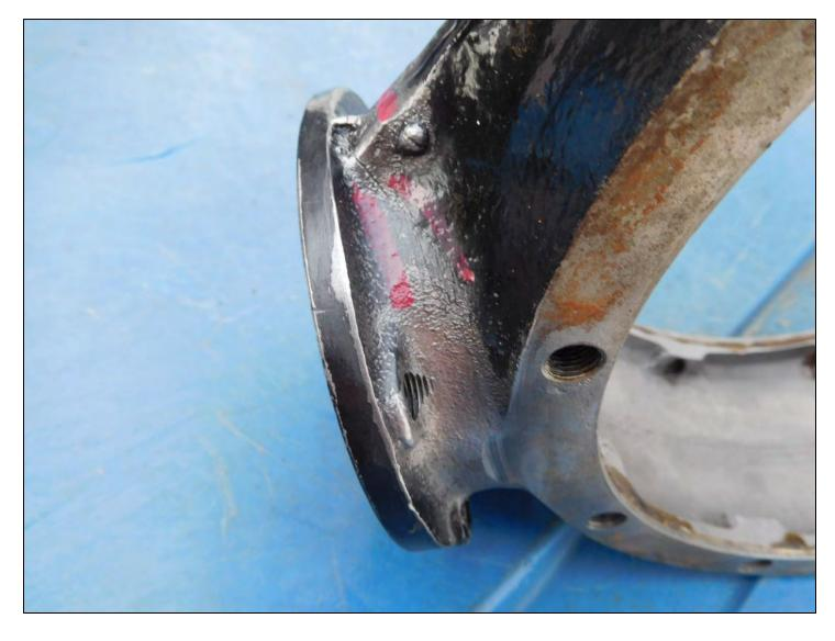
This photo shows a crack on the top left side of a 1930 banjo with support gussets that came out of my grandson's 1930 Tudor. The slot headed screw is a mystery and appears to have been included during the original casting of the banjo.
