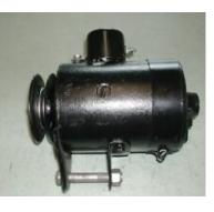
to open. An oil cup is provided for the rear bearing. It will be necessary to remove the rear cover of a Power House Generators to oil the rear bearing. Alternators have sealed bearings that do not require attention.
