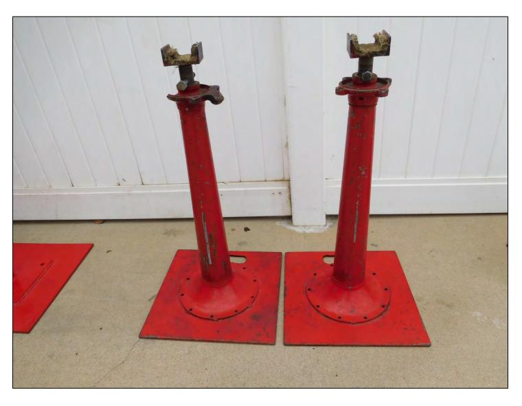
The rear jack stands were made from two discarded Model A axle housings welded to steel plates to provide a large footprint. Part of the wheel bearing surface was machined off. Ubrackets were welded onto steel shafts that insert down into the top of the axle housings. A hole was drilled through each shaft and a bolt is inserted through the hole to raise the Ubracket up.
