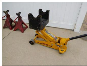
The jack fixture is constructed of wood with metal support brackets. It fits around the banjo on the rear axle. The jack has been modified with a large nut welded to the bottom of the raising platform. A large bolt goes down through the fixture to lock it in place on the jack.
