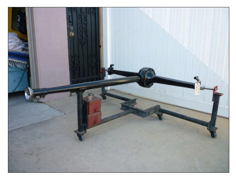
Another very handy tool is the rear axle assembly cradle. It can be rolled under a car once it is up on the jackstands. The rear axle assembly is then unhooked from the car and lowered into the cradle and rolled out from under the car.
