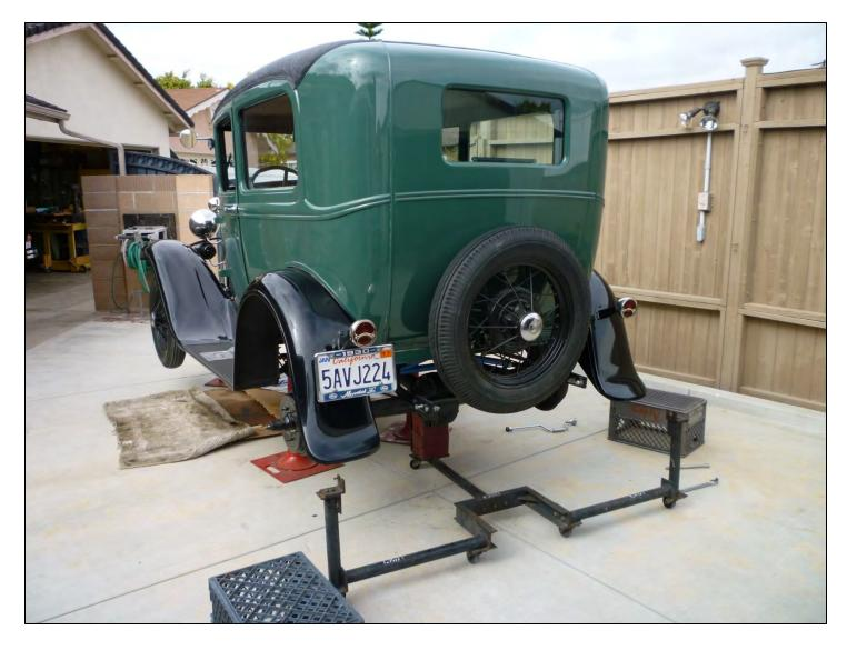
This photo shows a Model A Ford up on the jack stands ready for the rear axle assembly to be removed. The task is to install an overdrive. It can be seen that the rear brake drums are still attached to the rear axles. Only the rear wheels have been removed along with the axle nuts. The cradle will be rolled under the car and the rear axle assembly unbolted from the car and lowered into the cradle.
