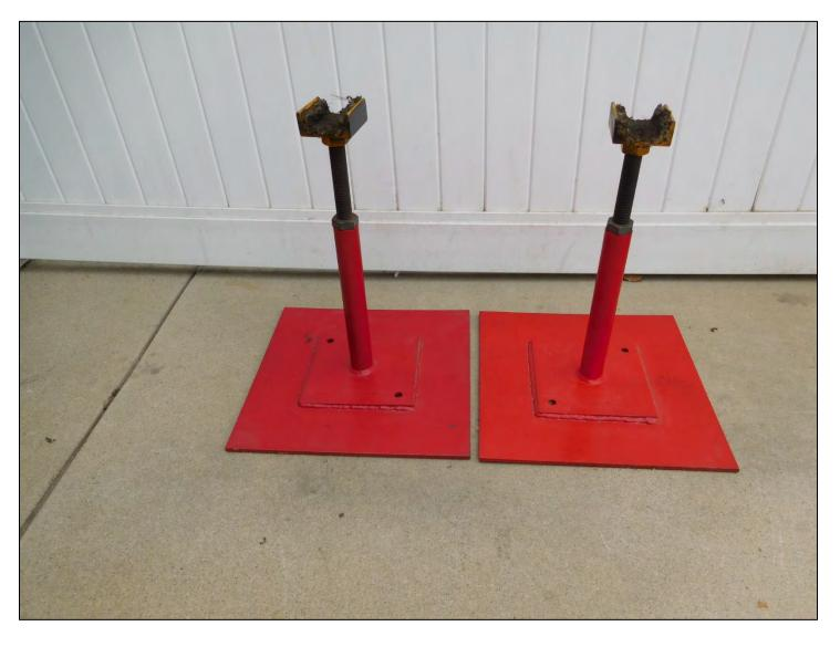
The front axle jack stands were fabricated and have U-shaped fixtures welded to the top of threaded steel shafts that are inserted into the vertical pipes. The front axle settles into the
