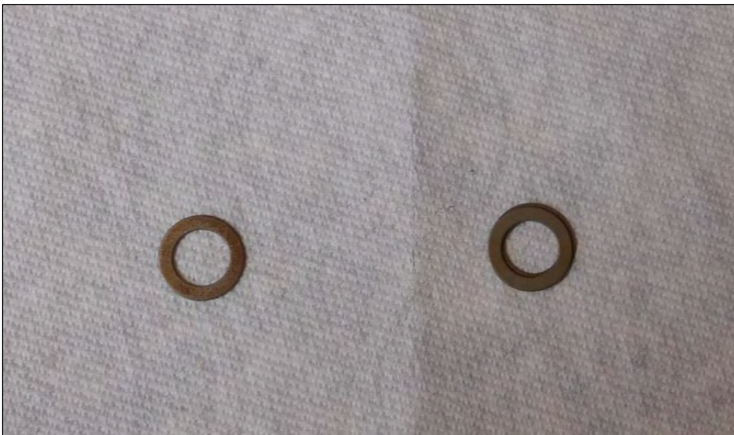
Shims used when installing the front radius rod bolts.
