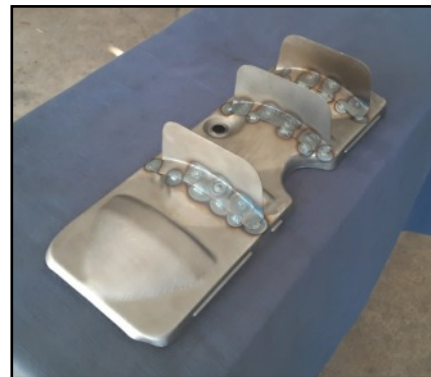
Cleaned parts with baffles re-welded.
