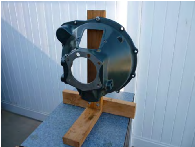
A simple wooden stand makes the assembly process easy. It can also be used for disassembly.
