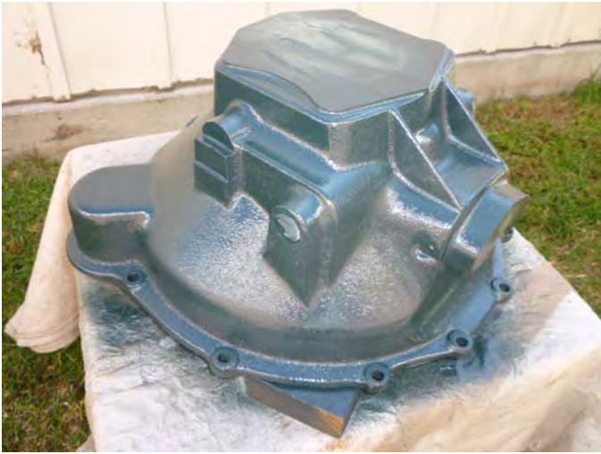
The machined surfaces are masked off and the outside of the bell housing is painted Ford green. The inside of the bell housing is left unpainted and sprayed with WD-40 to prevent rusting. The unpainted machined surfaces are also coated with WD-40.
