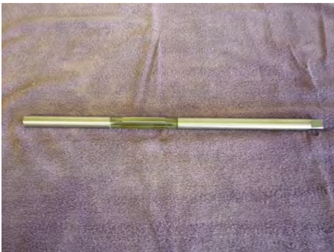
Bushing reamer. This tool is long enough to ream both bell housing bushings in line. It is also used to ream the pedal bushings.
