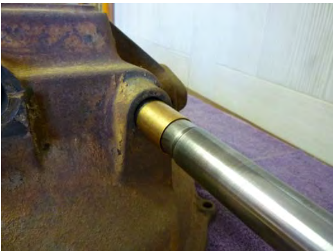
The bushing tool can be used to drive the old bushings out and to drive the new bushings into place.
