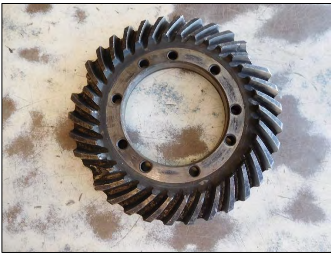
Teeth broken off the ring gear
