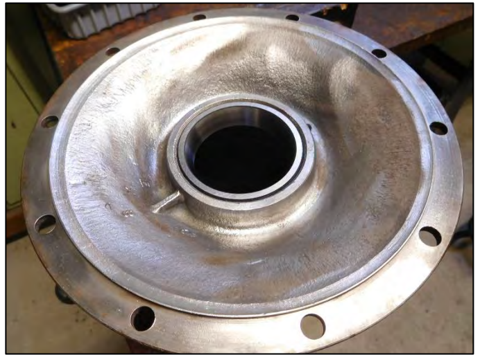
The inside of the axle housing should be smooth
