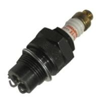
Good quality spark plugs spark. Model B cams are replacement for the Model A cam and are readily available. If your engine is in good condition and you drive your car on a regular basis, spark plugs should last 10,000 miles at a minimum. I have over 18,000 miles on the spark plugs in my Model A Tudor and they still less likely to fail due to the head
