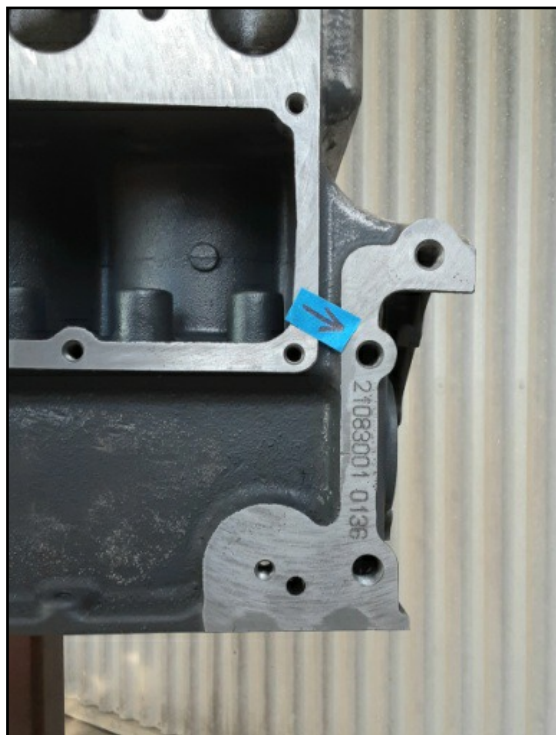
The arrow points to an oil passage hole that must be plugged and sealed by a 7/16-14 “set screw”.
