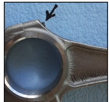
Arrow indicates where rod cap bolt protruded slightly.
