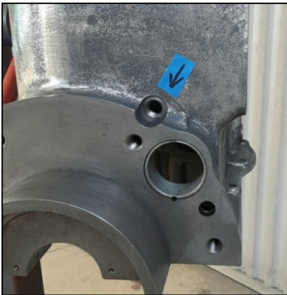
The arrow shows where a 1/2 inch long, 1/2-13 socket head cap screw (Allen screw) with an aluminum sealing washer was installed.
