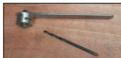
Special tooling to drill cam bearing shells
