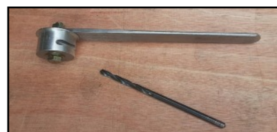
Special tooling to drill cam bearing shells
