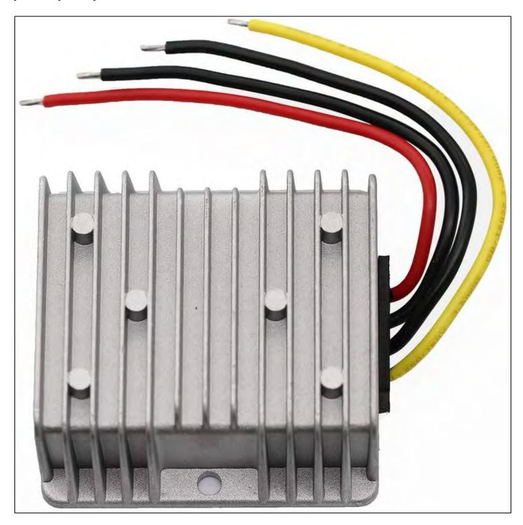
The converter is available on-line from Amazon and is described as a Digiten 6-volt to 12-volt converter with a 10 amp output capacity. The device size is 2.9" X 2.9" X 1.25" and is priced at \$28.99.
