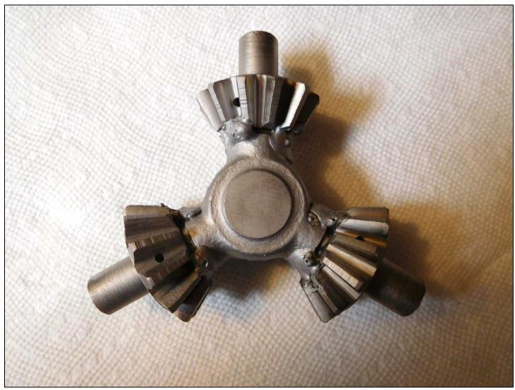
The poor man's Posi traction that came out of Model A Ford that was one time owned in 1950 by a 17 year old kid with a duck tail haircut.
