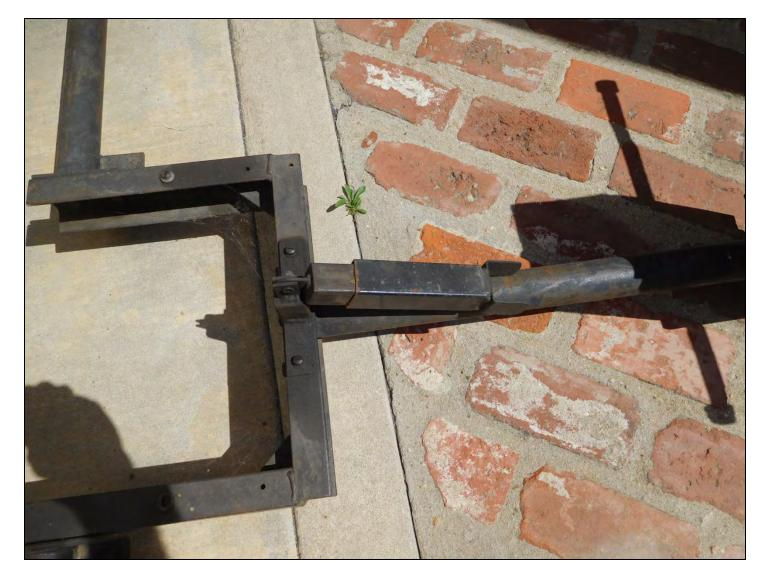
Another modification is the device seen folded over at the front of the U-section. Its purpose is to provide a support for the Mitchell overdrive stub shaft after it is installed. This is used when the cradle is being used without the radius rods installed on the rear axle assembly.
