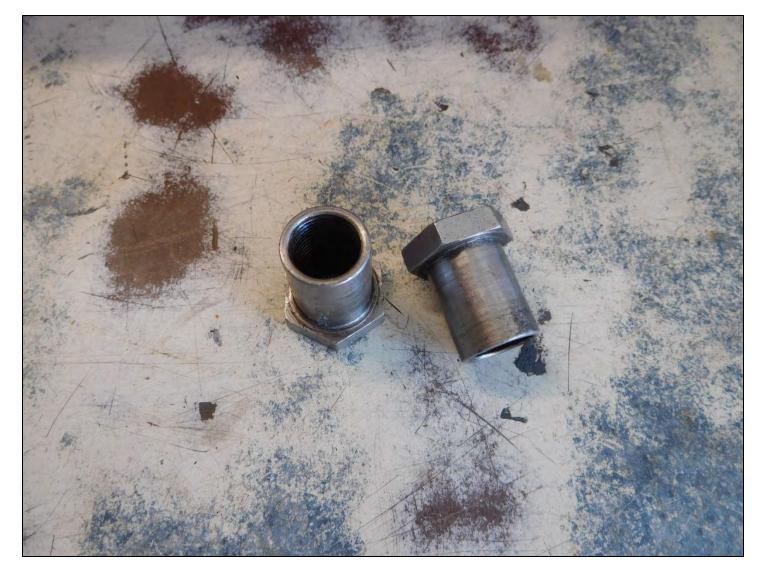
These two devices were machined to screw over the threaded ends of the axle shafts to protect the threads. They also lock the axle housing in place and provide a means to pull an axle housing off one side without pulling the whole rear axle assembly out of the cradle. The cradle provides a platform to disassemble a complete rear axle assembly after it s removed from the car.
