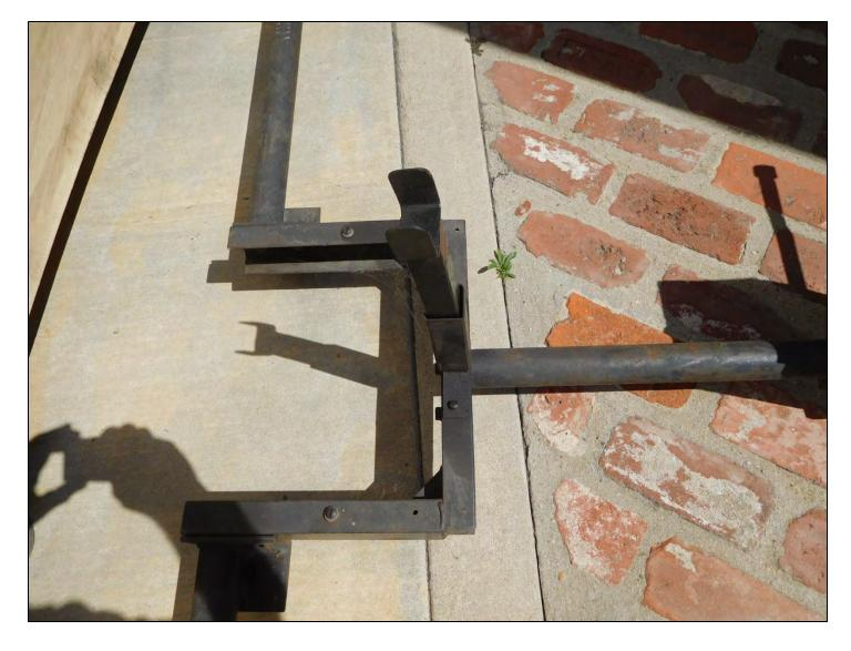
The stub shaft support is shown in the upright position.
