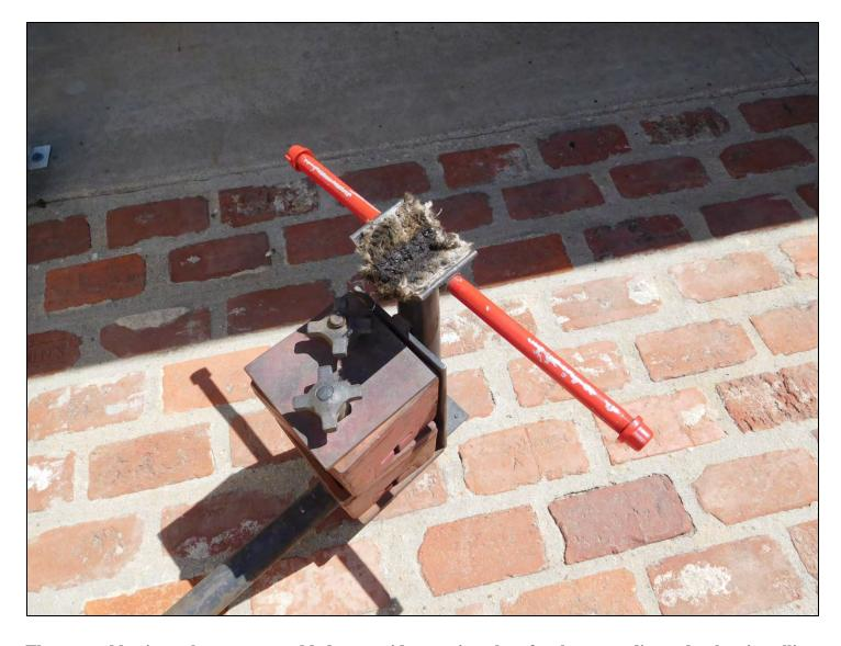
The two red horizontal struts were added to provide a resting place for the two radius rods when installing a Mitchell overdrive. During the installation the rear axle assembly remains in the cradle and only the torque tube and drive shaft are removed. The radius rods are then allowed to rest on the struts keeping them level and preventing oil from spilling out of the banjo.
