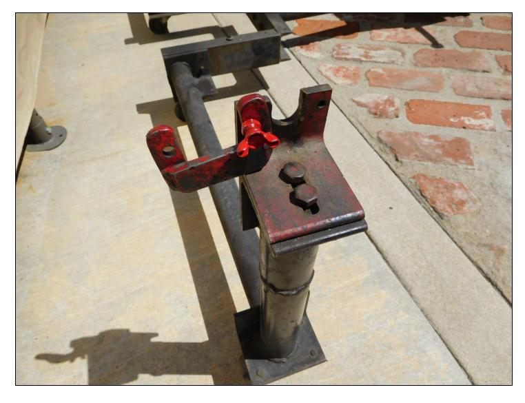
Shown here is the device used to secure the threaded end of the axle to the support. Also shown is how the support can be moved laterally to accommodate a rear axle assembly with or without brake drums attached. The U-shape cap attached to one side pivots over the threaded end of the axle and is bolted on the other side.
