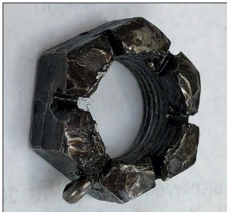
The damaged drive shaft nut
