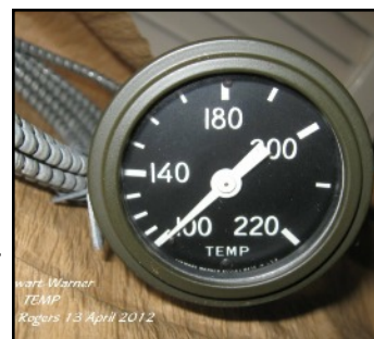
Mechanical temperature gauge with a 270 degree "sweep" dial
