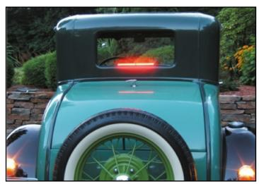
Another improvement is the addition of additional tail light assemblies and also red reflectors. Reflectors are very effective when driving at night.
