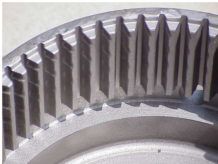
Notches worn in the flywheel
