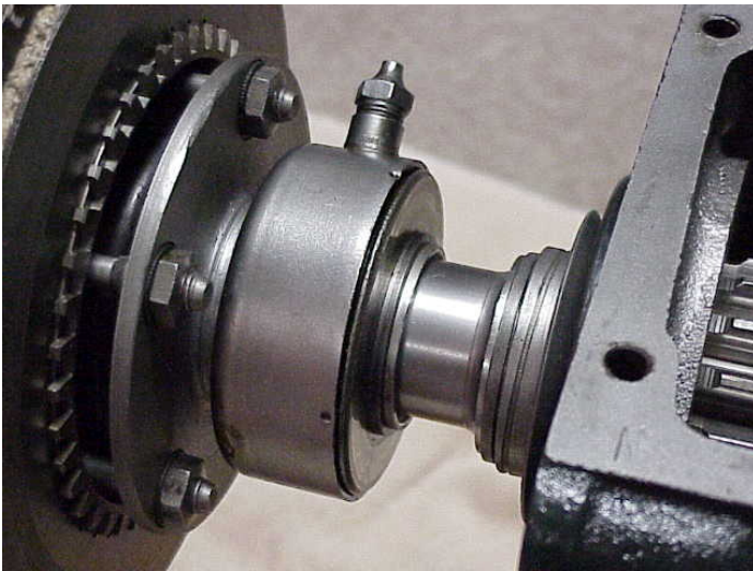
The throw-out bearing and extra oil baffle
