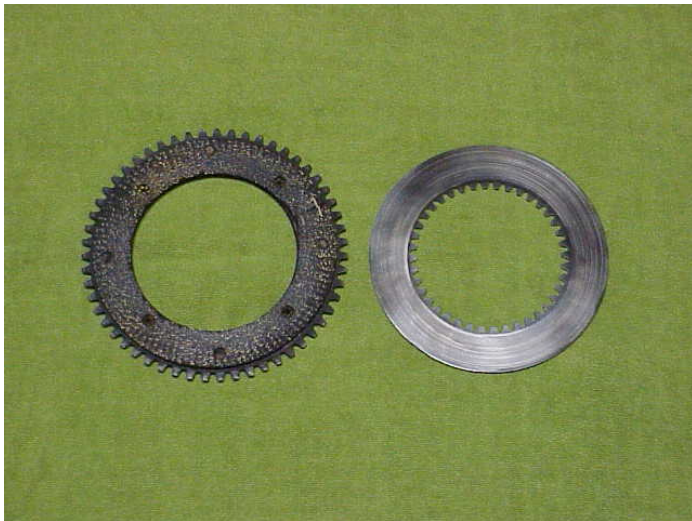
Driving disk (left) driven disk (right)
