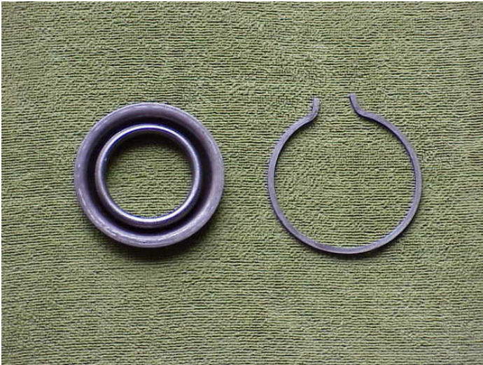
A7047-R oil baffle and A7046-R snap ring
