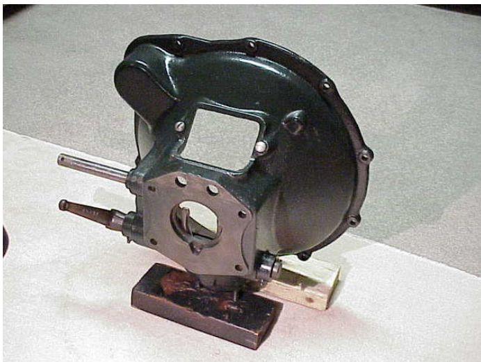
The multiple disk clutch bell housing
