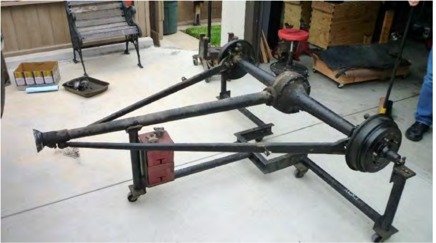
The rear axle assembly has been removed from the car. The torque tube is ready to come off. The rear spring is still attached to the frame of the car with the spring spreader still installed.
