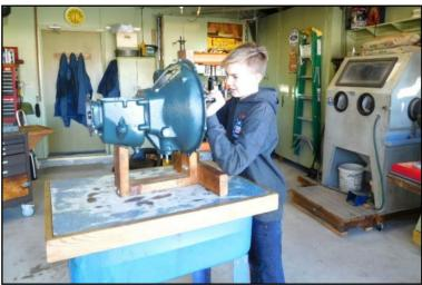
The photo on the left shows a Model A Ford undergoing a Mitchell overdrive installation. The photo on the right shows Ben Stone attaching a Mitchell synchronous transmission to a bell housing.
