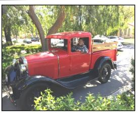
The serial number is not known but it has a steel top cab manufactured by the Budd company. That means it had to be produced in September of 1931 or later. The car had a B engine in it and ran OK but I replaced it with another B rebuilt engine. I fixed the brakes and steering, added the wood side rails and switched to 16" wheels.
