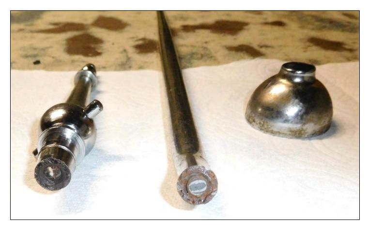
The best option is to always use an original gearshift lever, and one that is bent to the correct angle for your year car. The worn ball on the end of the lever can be welded up and ground down to fit the slots in the shifting forks. Quite often the issue is that the plating is shot and having something re-plated in the US is sometimes very difficult. The original gearshift levers were plated in what is known as a "Butler" finish, that had a dull appearance.
