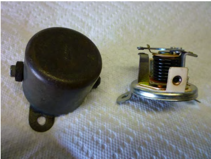
Original quality Ford cut-out on the left. Insides of a poor-quality reproduction on the right
