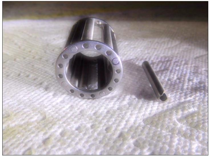
Note the protrusion stamped into the end plate at the rear. Note that what appears to be holes in the end plate at the front are not holes, but are the inside of the protrusion. Note the element on the right, there is a recess drilled into each end. The element end was broken during the process of removing it from the bearing.
