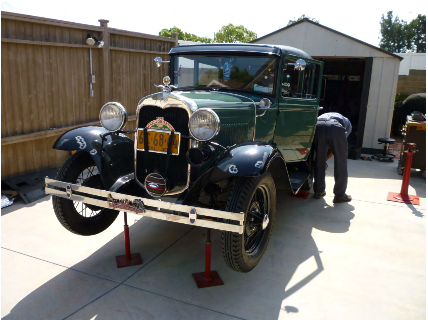
The car is put on jack stands and the rear wheels removed
