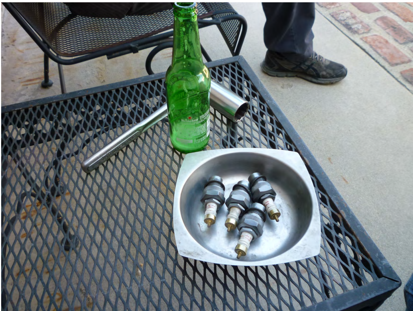
The 3X spark plugs were cleaned and re-gapped during a beer break
