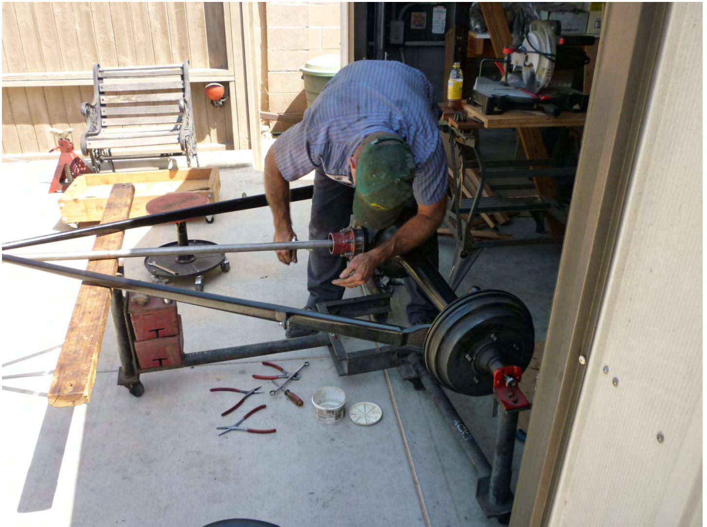
The pinion puller-inner tool is being installed
