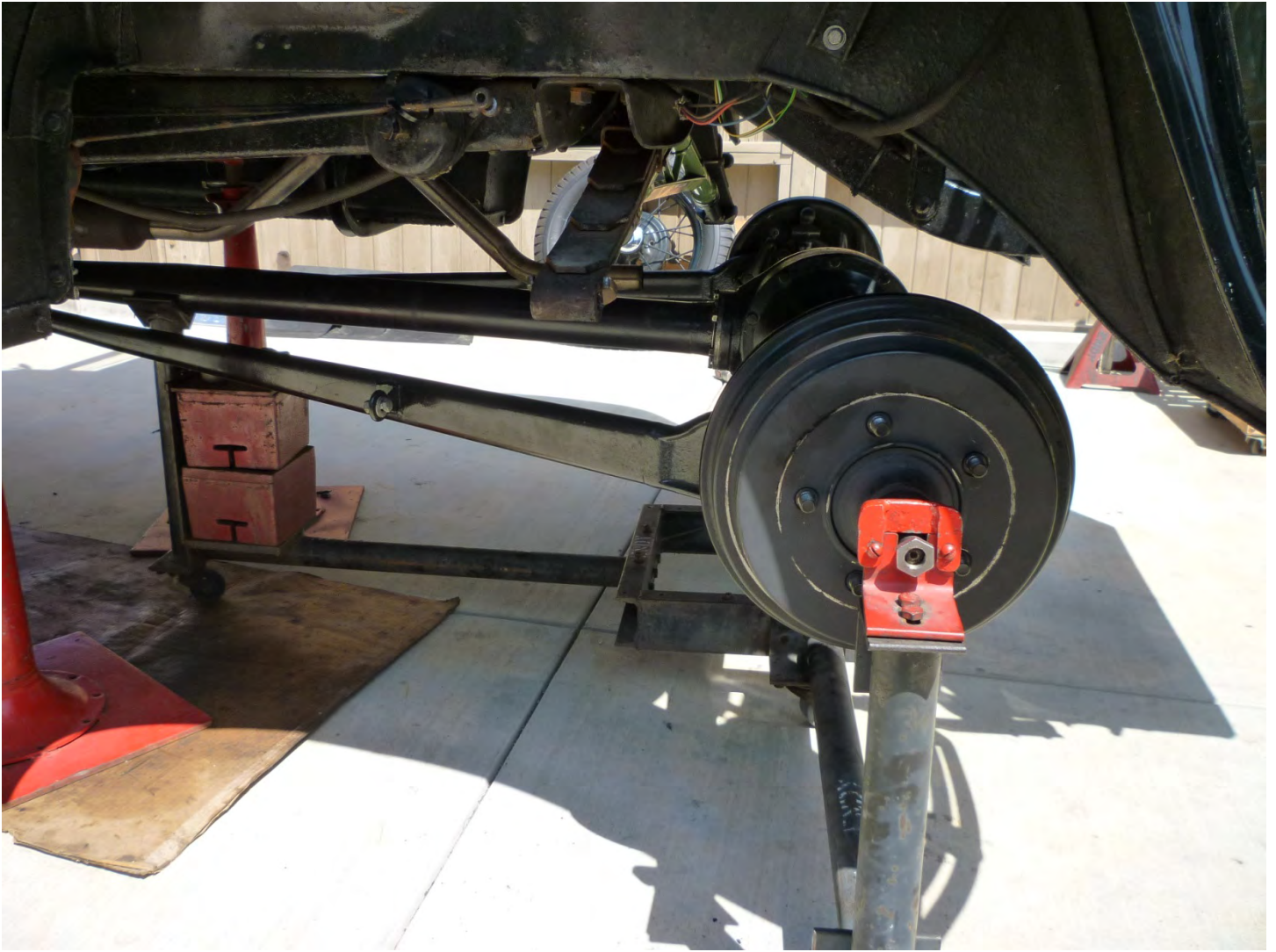
The rear axle assembly minus the overdrive is being installed back into the car
