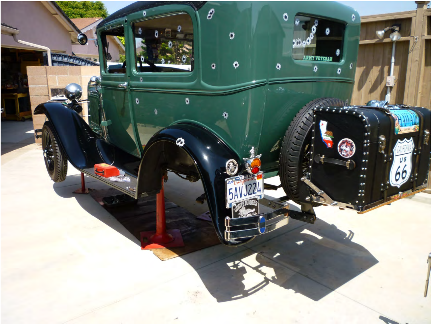
The rear axle assembly with the overdrive has been removed from the car
