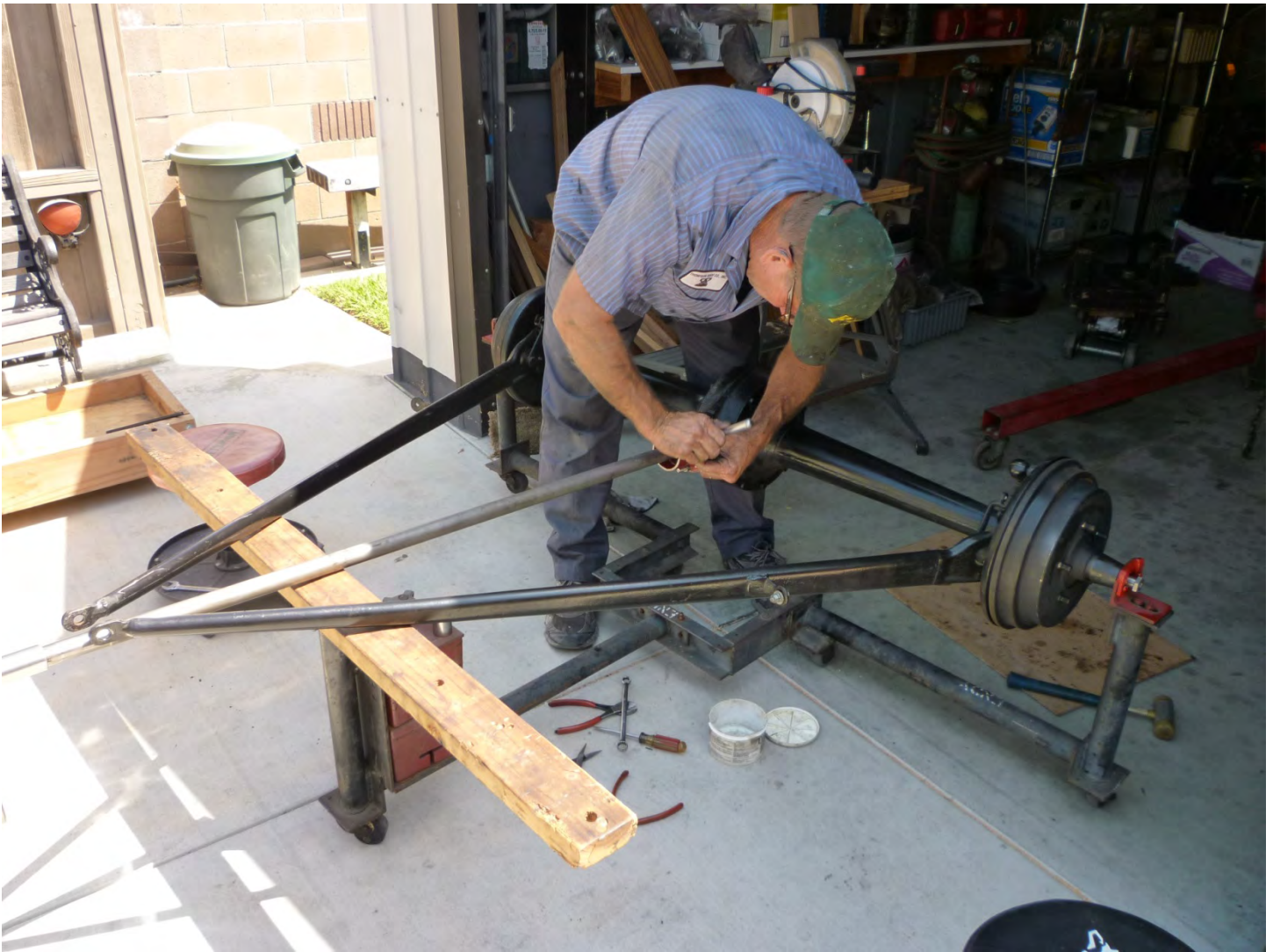
The overdrive and stub shaft have been removed and are replaced with a drive shaft
