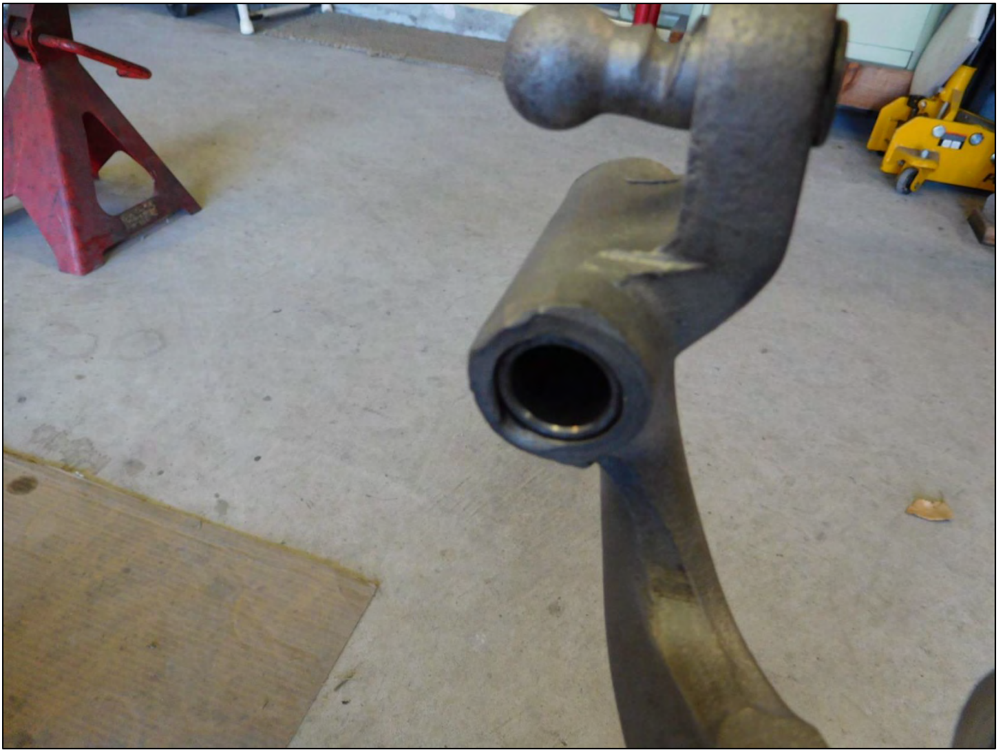
New shackle bushings have been installed.
