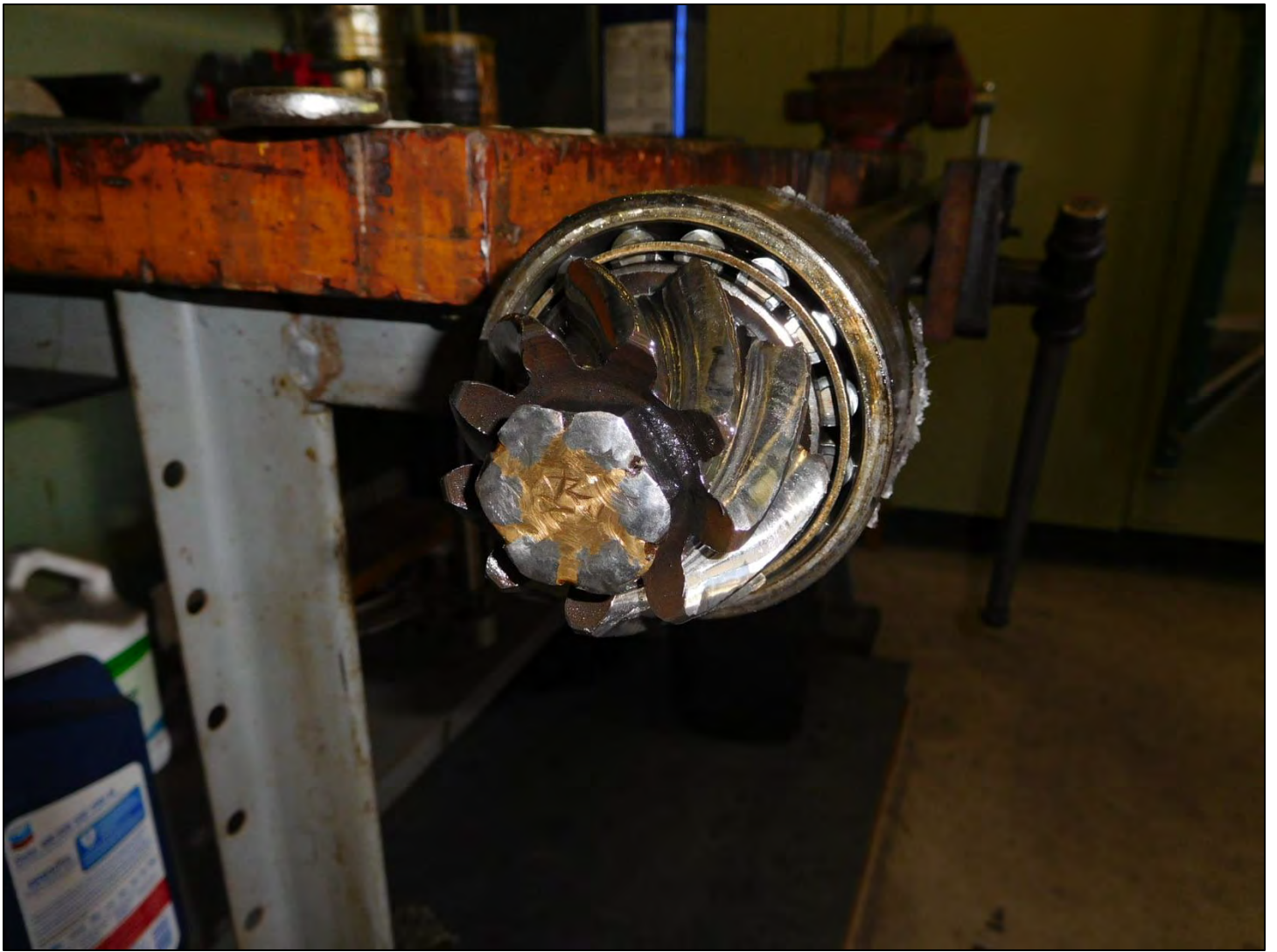
The nut on the end of the drive shaft is seen here braised onto the end of the drive shaft.
