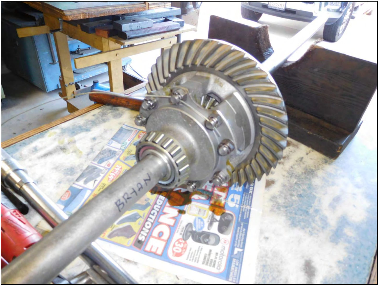
The two replacement axles have been installed in the carrier assembly and it is being safety wired.
