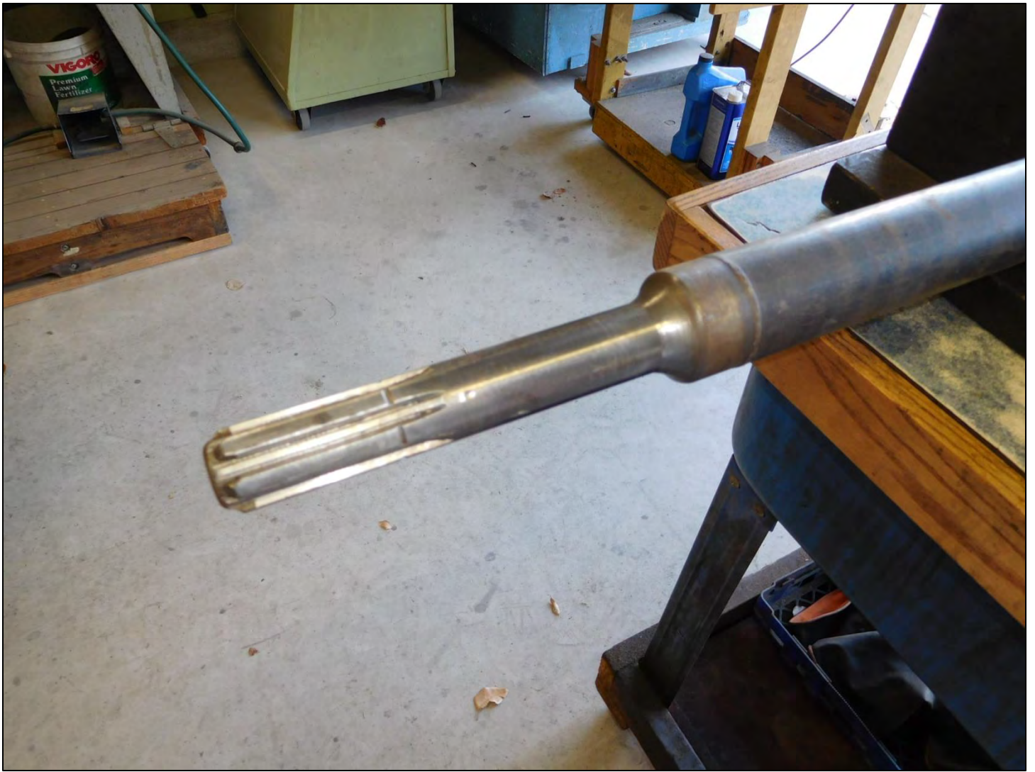
The bearing race surface and spline of the drive shaft are in excellent condition.
