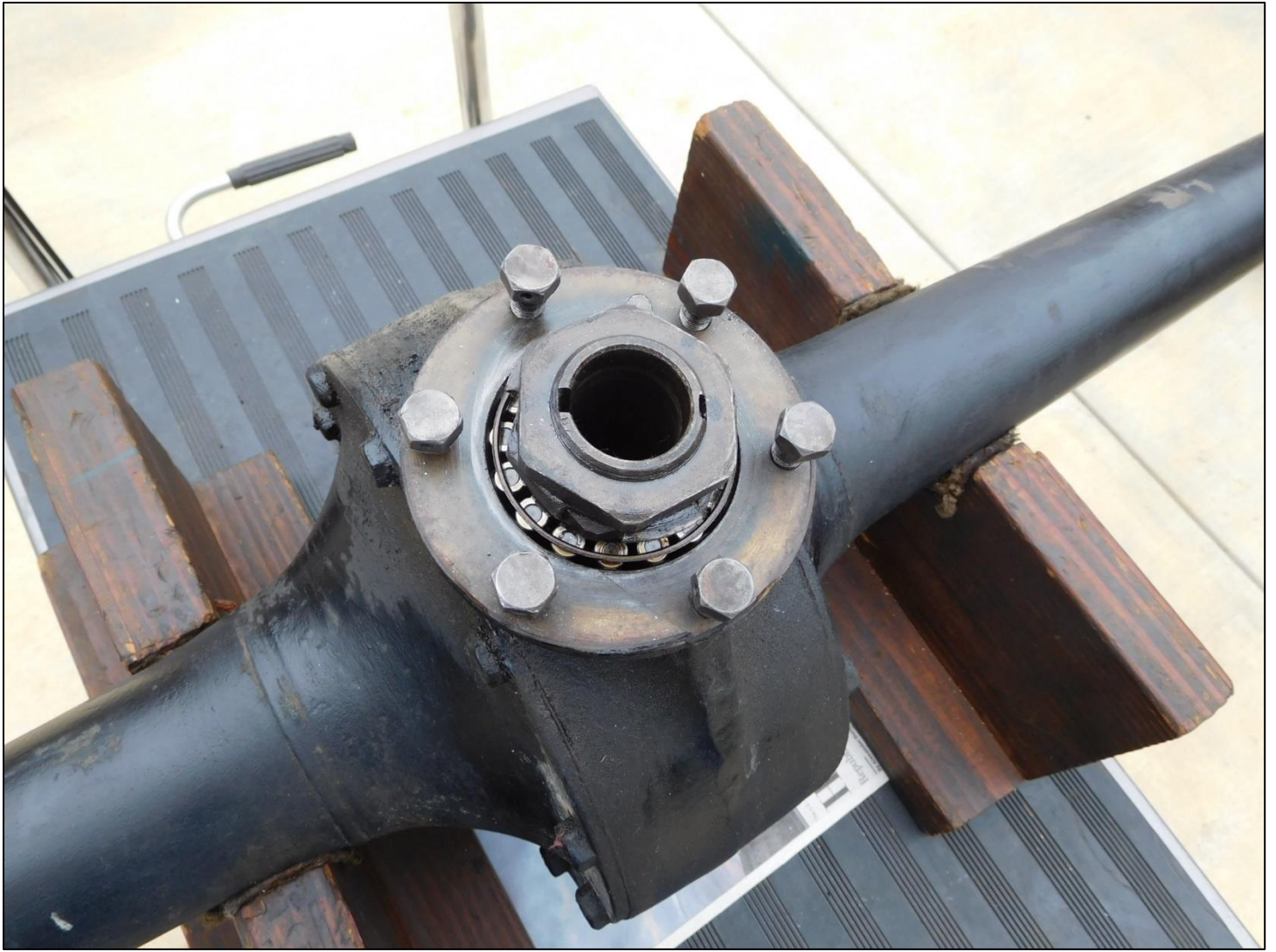
A close-up photo showing where the Borg Warner stub shaft should be protruding from.
