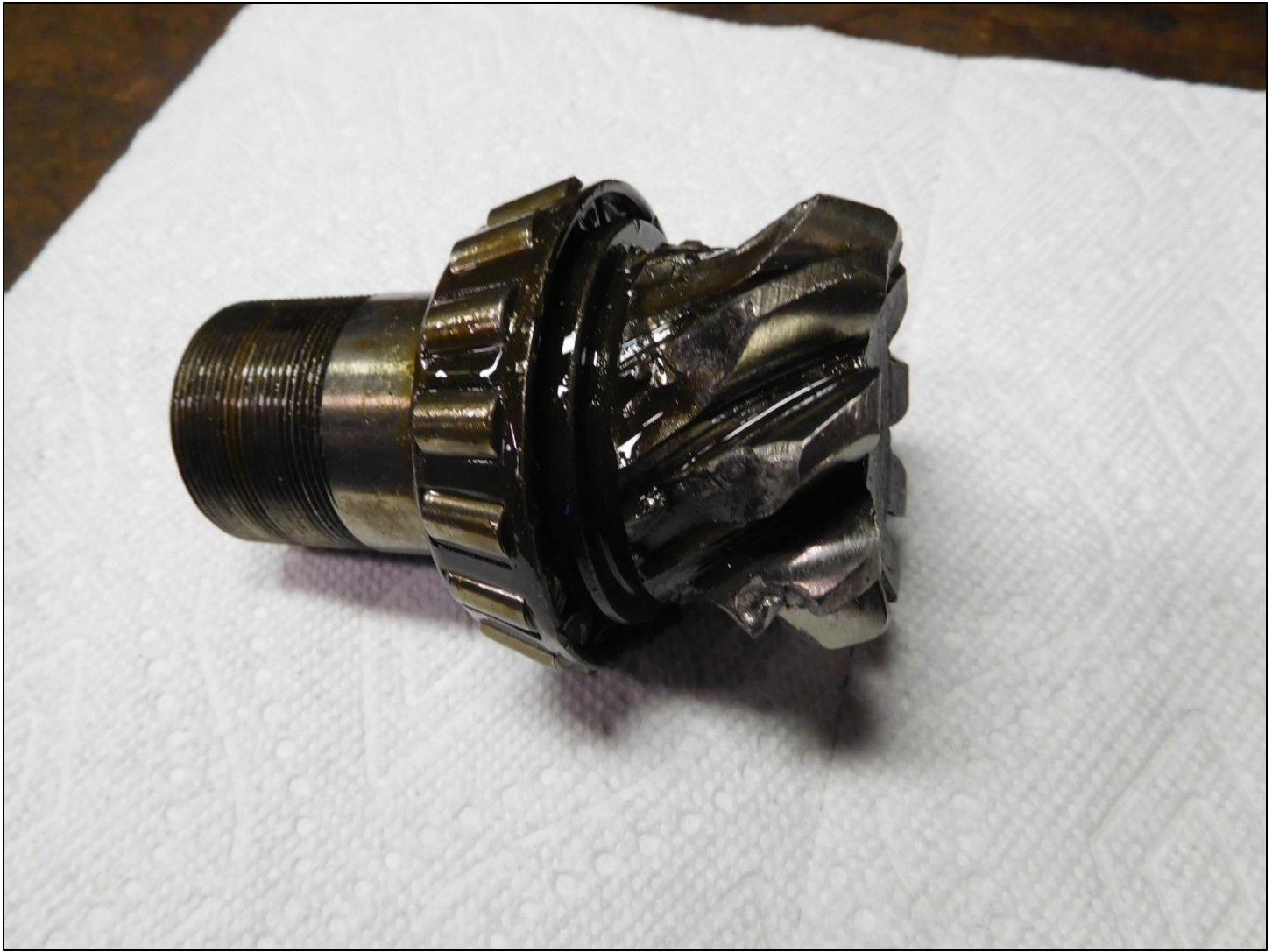
Shown here is the damaged pinion gear. Note the many teeth missing from the gear.
