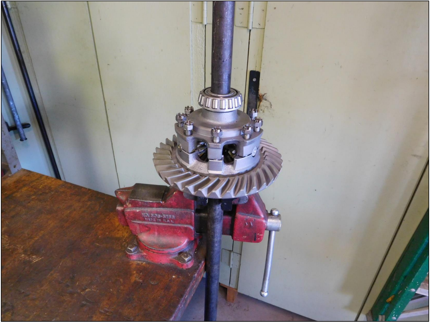
The two axles along with the spider gears are shown here being assembled into the carrier.
