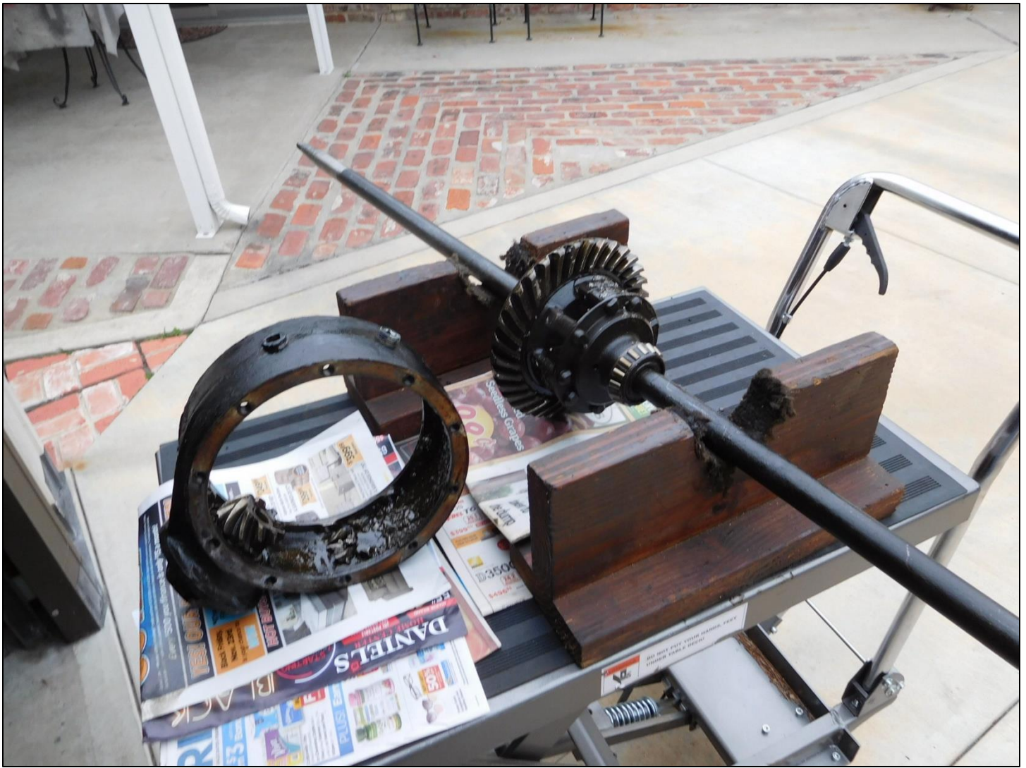
This photo shows after the two axle housings were removed: The banjo with the pinion gear still installed and the carrier assembly with the two axle shafts still installed. Note the metal debris in the bottom of the banjo.
