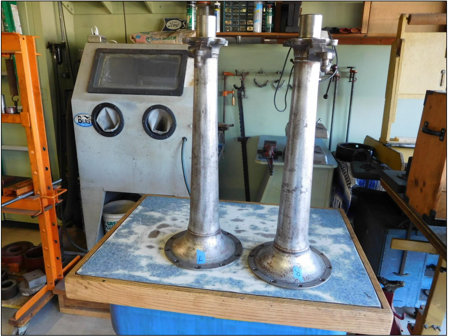
Both axle housings have been cleaned up, new races and seals have been installed.
