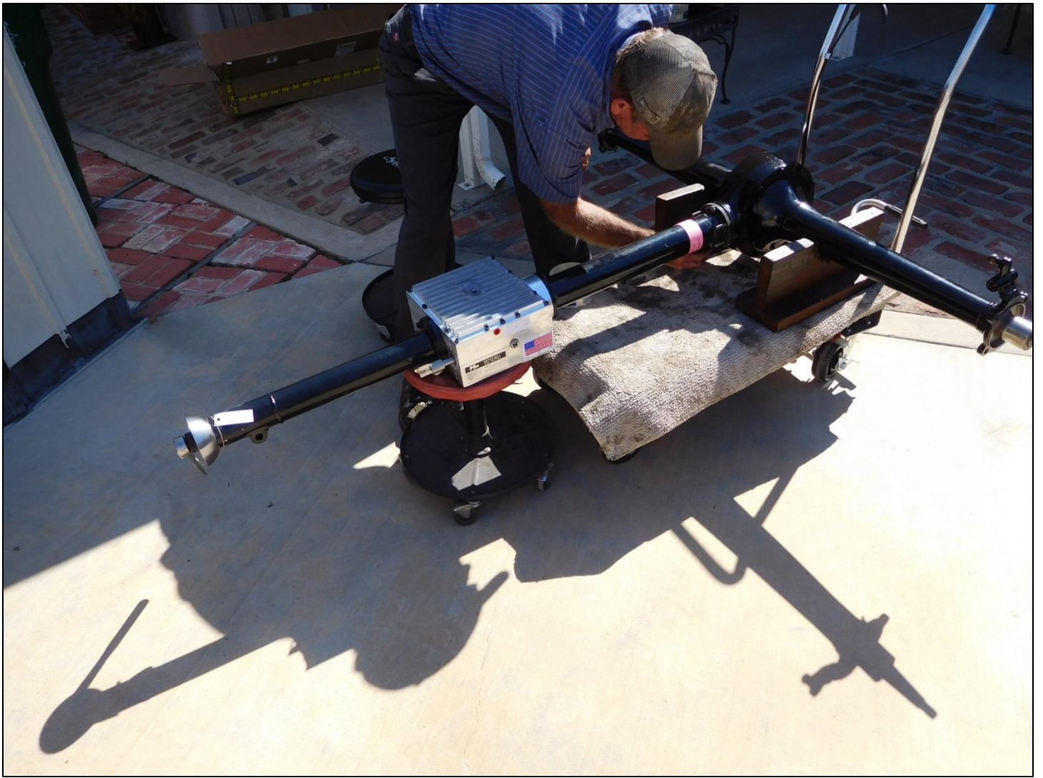
The Mitchell overdrive arrived and is shown here being installed onto the overhauled rear axle assembly.
