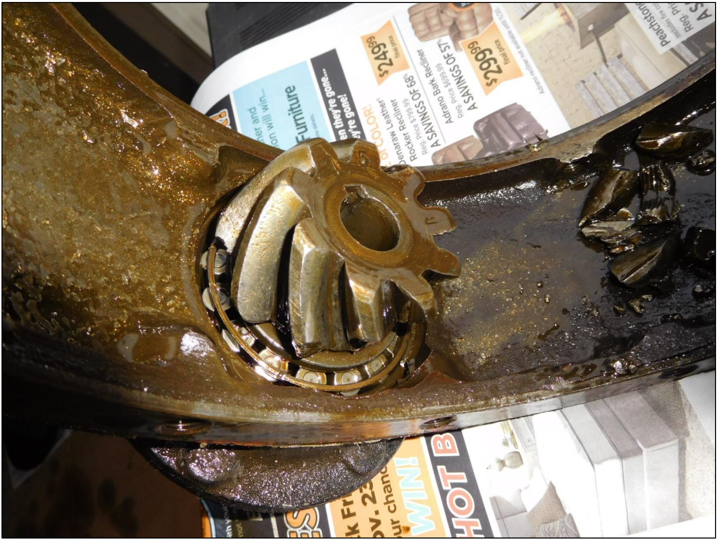
This photo shows the pinion gear with the nut missing from where the threaded end of the stub shaft would have protruded and secured with a nut and cotter pin. Note the broken teeth from the pinion gear in the bottom of the banjo.
