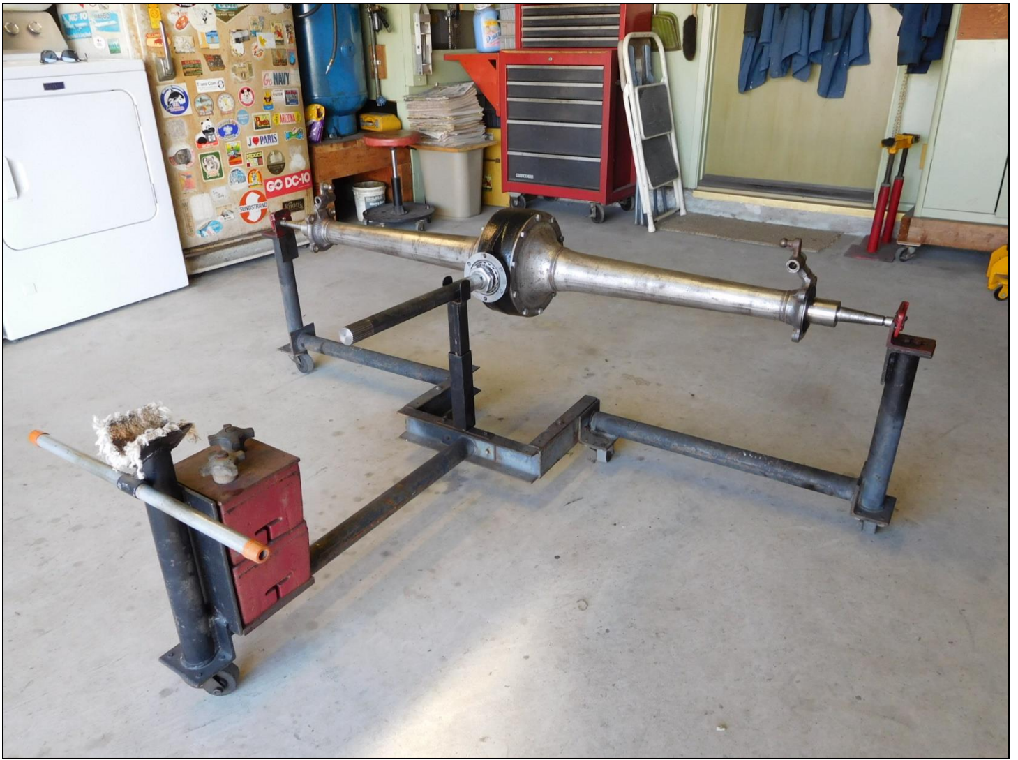
The rear axle assembly is complete and the housings have been sanded. The next step is to paint it.
