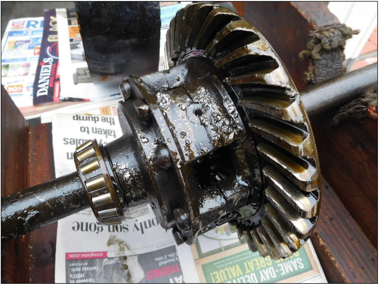
Shown here is metal debris from the pinion gear scattered on the carrier assembly. The teeth on the ring gear are also battered.
