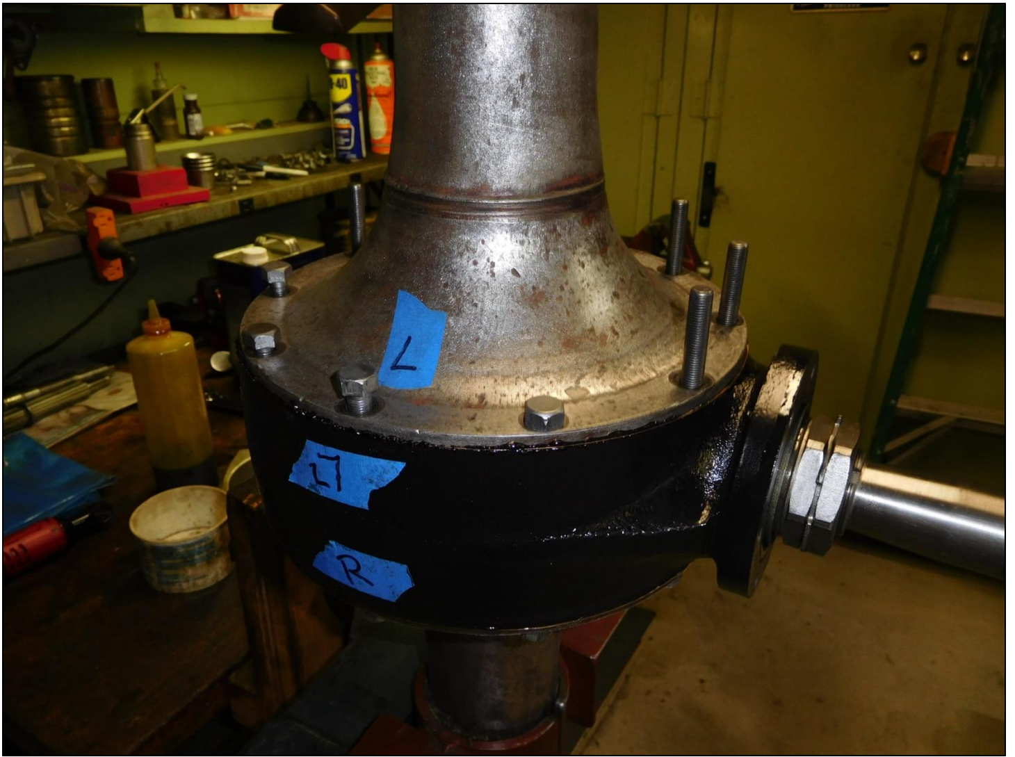
The 20 banjo bolts are torqued to 35 ft. lbs.
