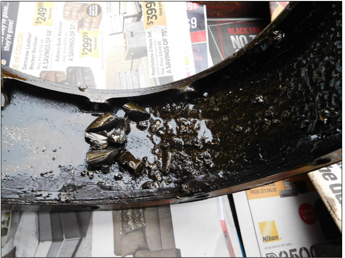
Close up of broken teeth from the pinion gear in the bottom of the banjo.
