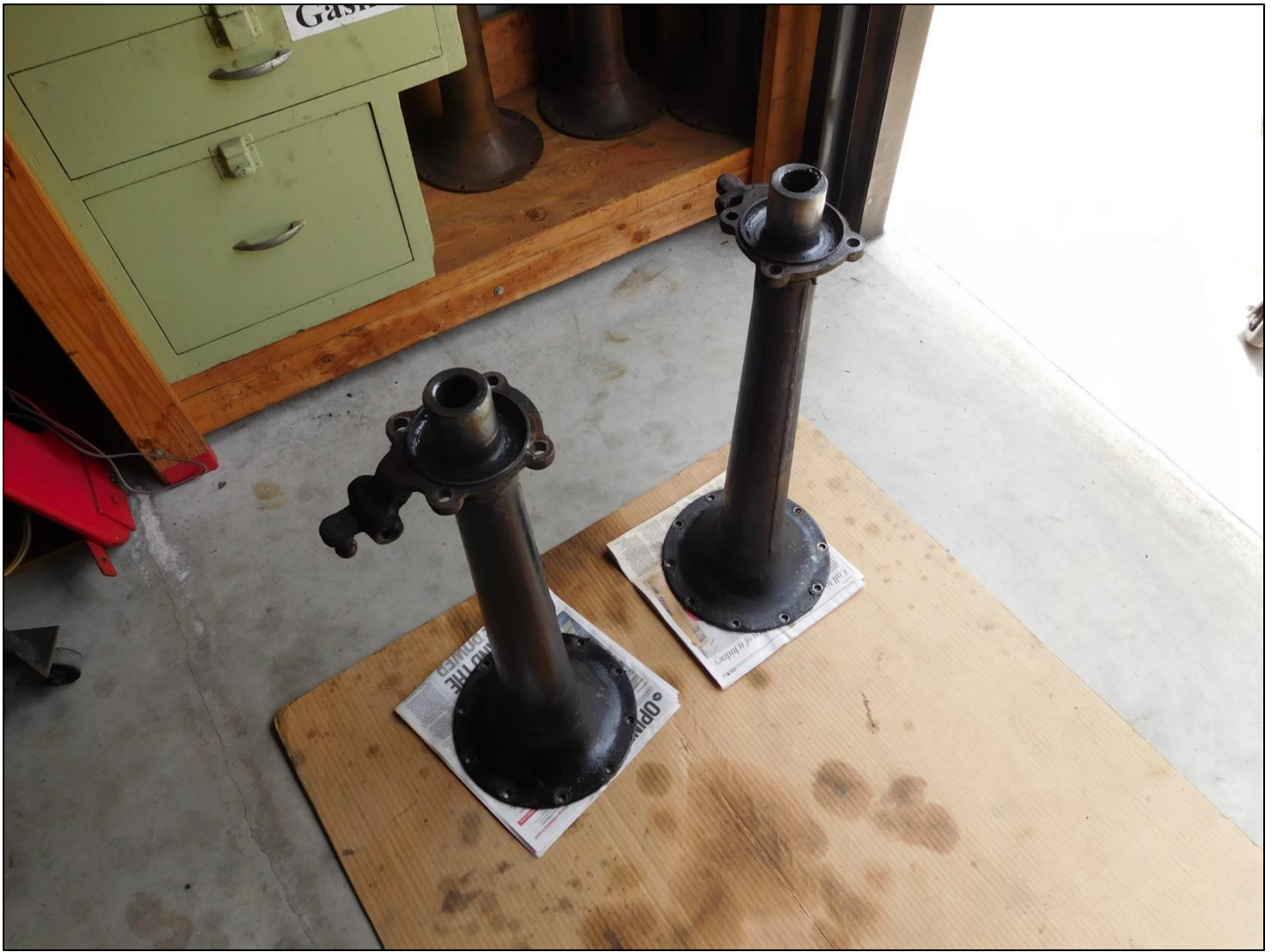
The two axle housings have been removed. The grease seals and the carrier bearing races have been removed and the housings are ready for clean-up.
