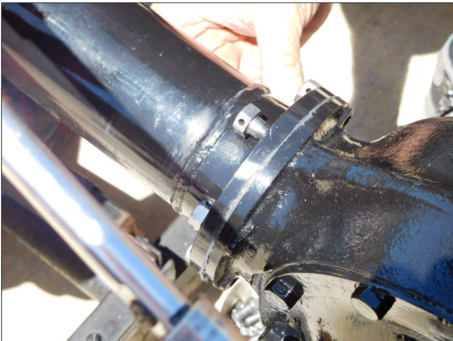
The six mounting bolts secure the overdrive to the banjo and are safety wired.
