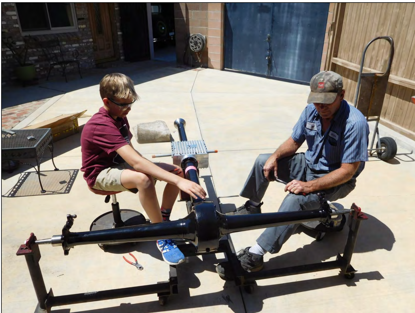
Ben and Bryan have installed the overdrive onto the rear axle assembly.
