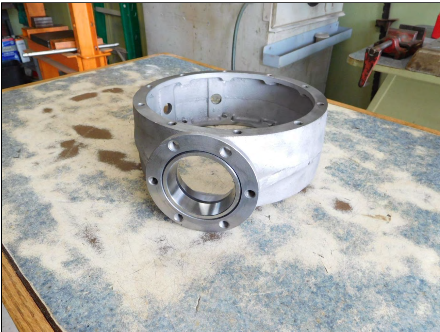
Shown here is the banjo with a new pinion bearing race pressed into place.
