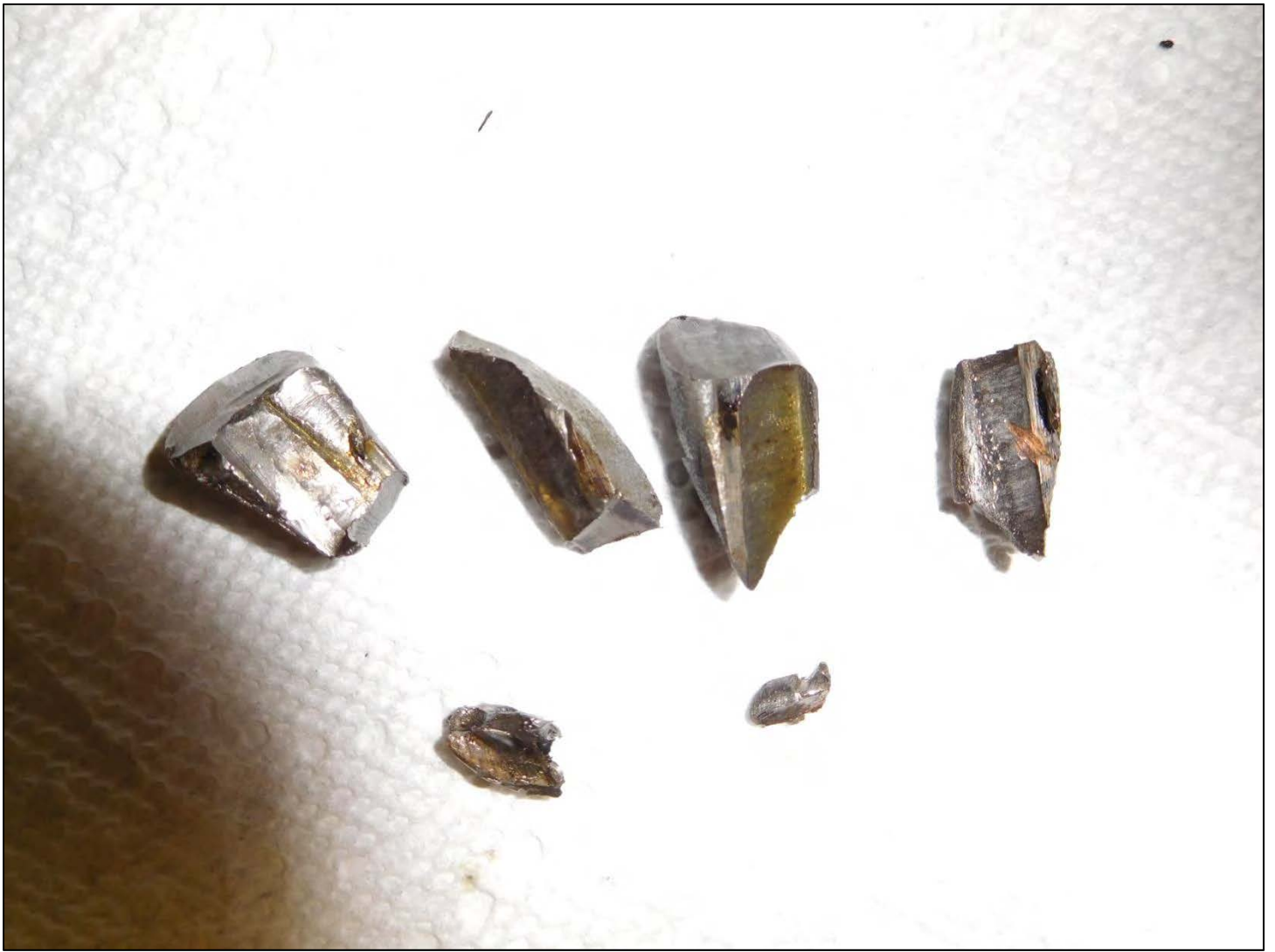
Teeth broken off the ring gear were found in the bottom of the banjo.
