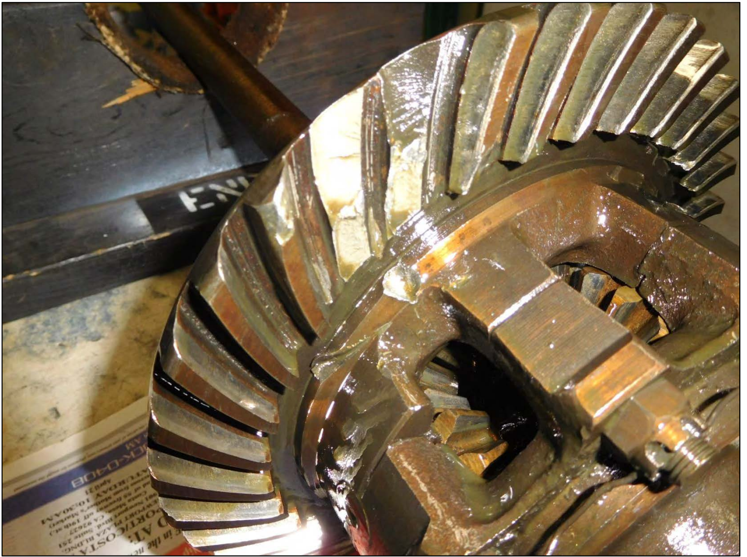
Close up view of the damaged area of the ring gear.
