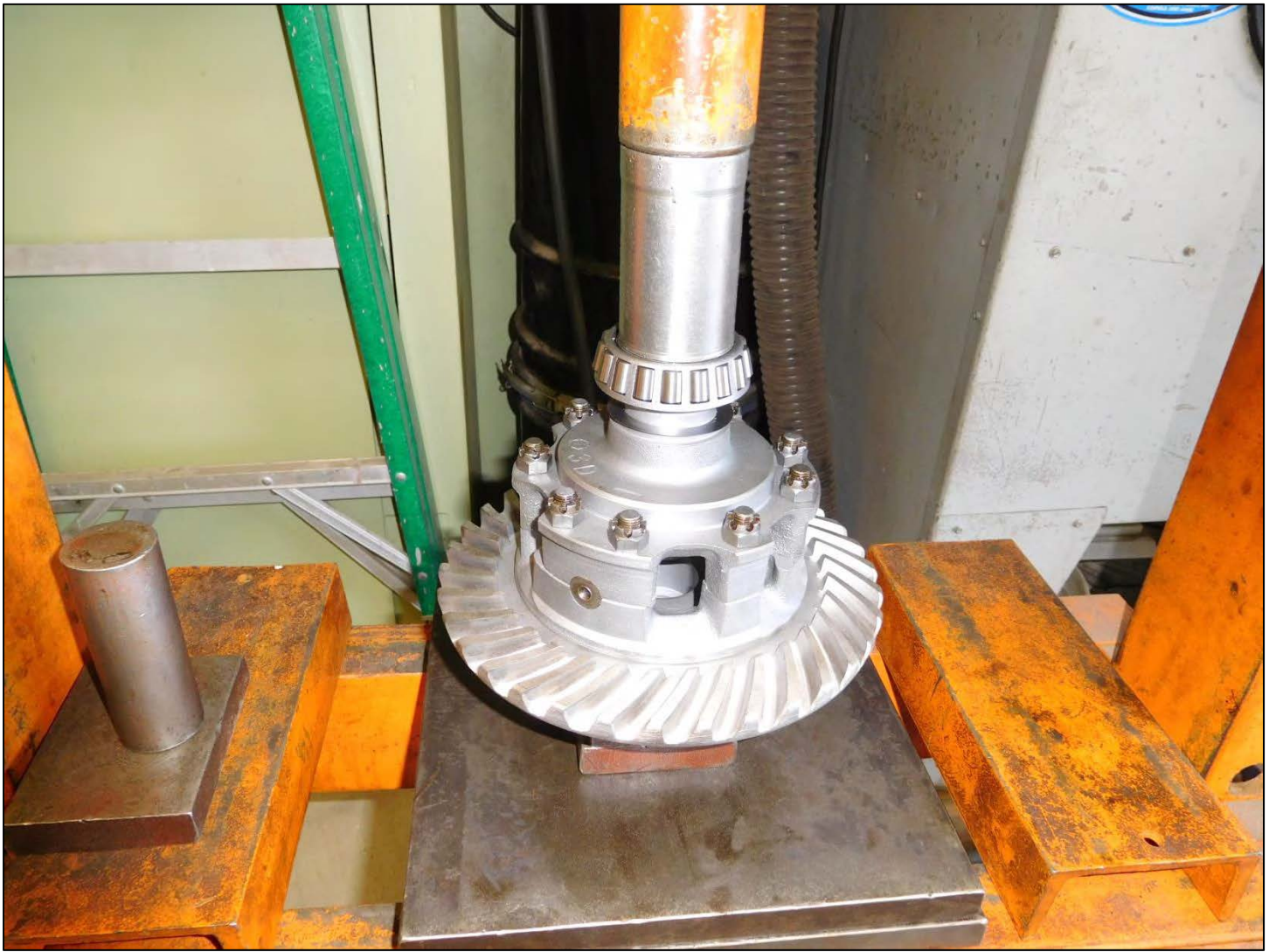
The bearing is being pressed down on top of the shim.
