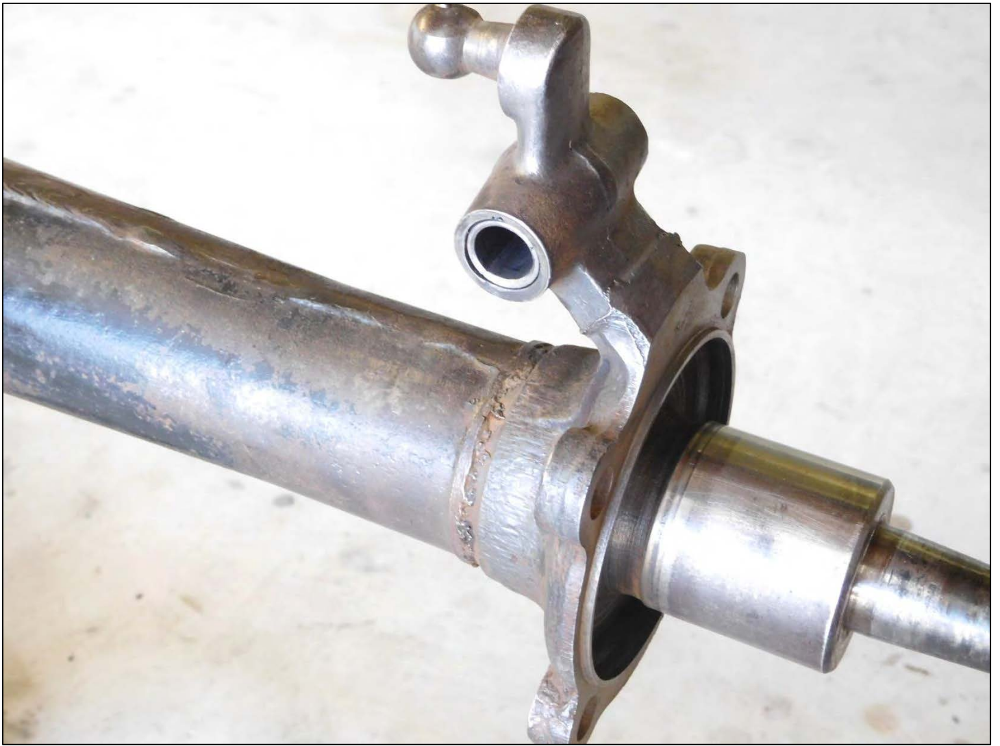
New shackle bushings were installed in both axle housings.
