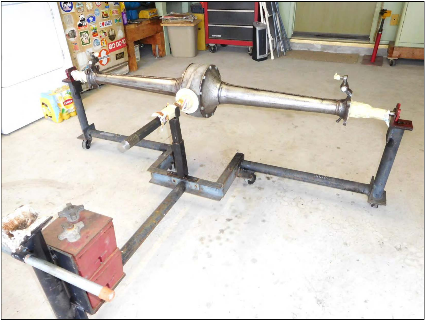
The rear axle assembly has been masked off and sanded and is ready for painting.
