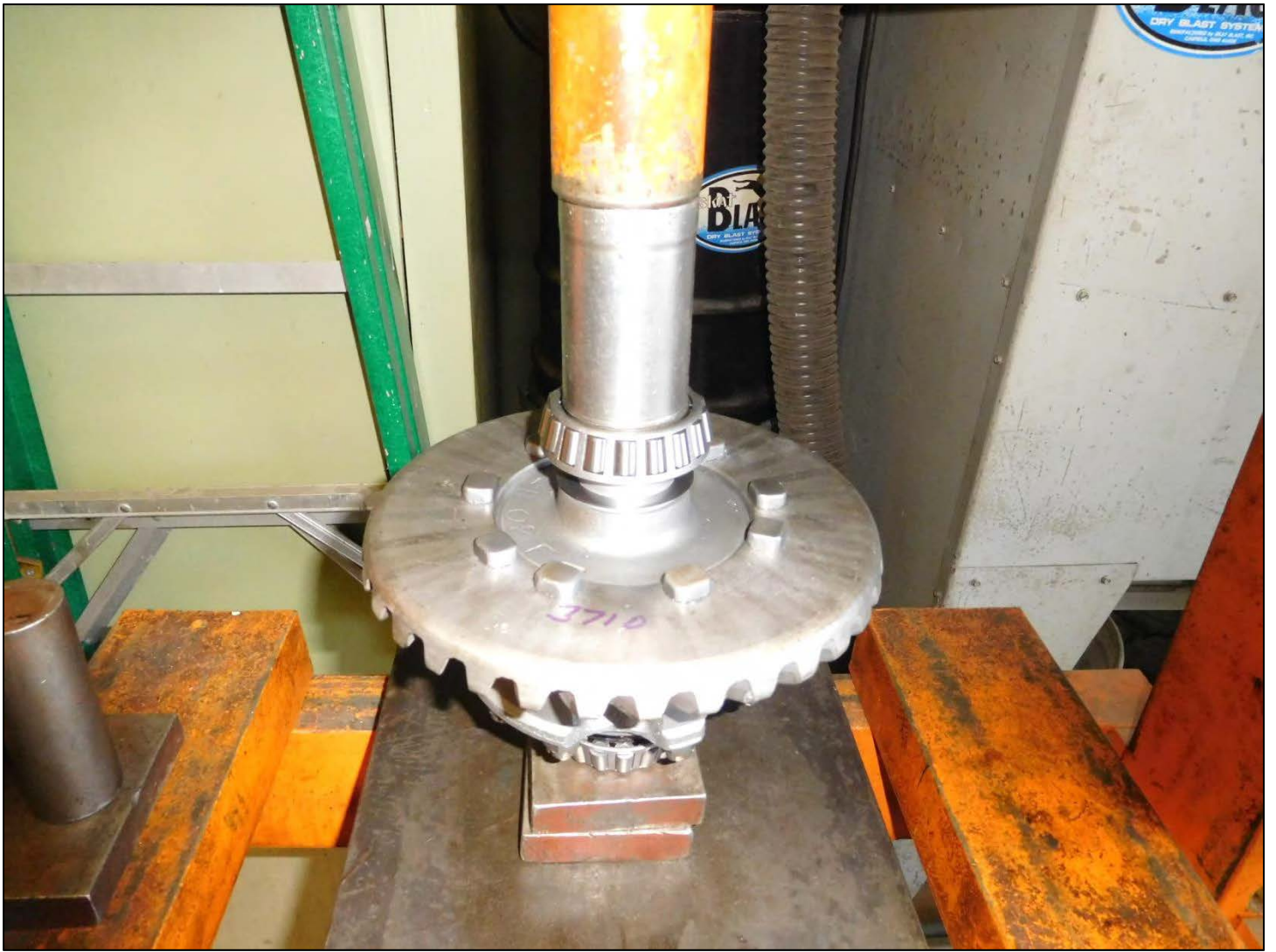
The other bearing is being pressed on.
