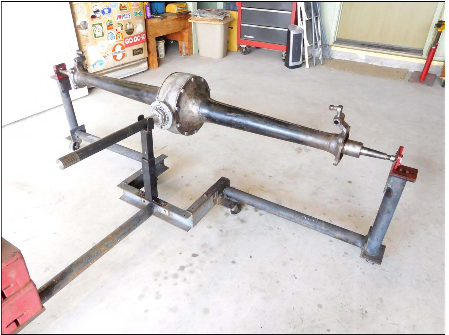
The rear axle assembly is complete and has been put back in the roll around cradle.
