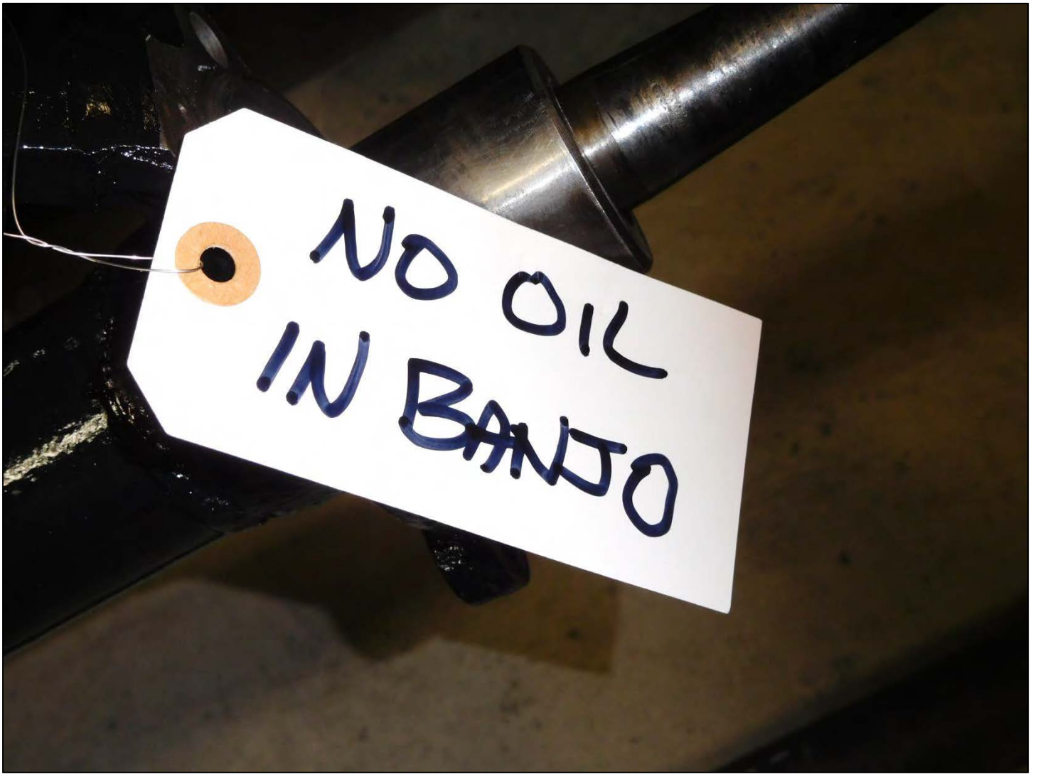
Tag attached to the rear axle housing. Don't forget to put oil in the banjo.
