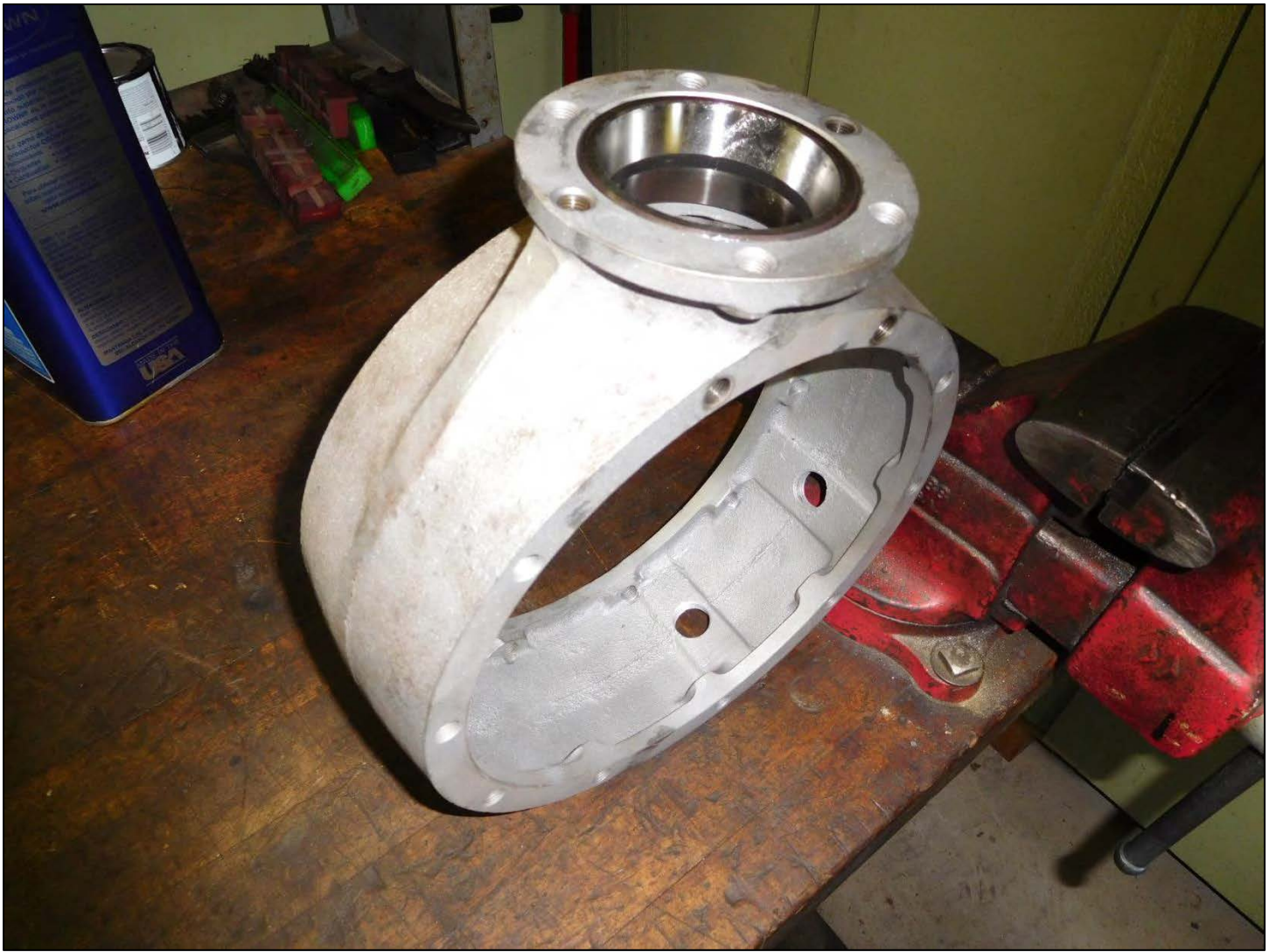
The banjo was degreased and bead blasted. A new double race was pressed into place.
