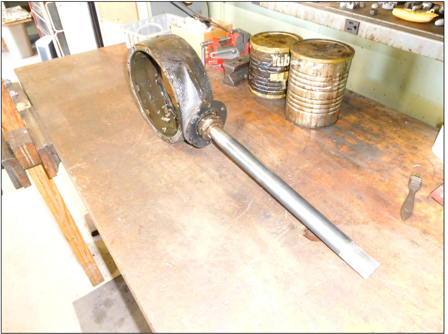
The banjo shown with the Mitchell stub shaft installed. Broken teeth from the ring gear can be seen in the bottom of the banjo.
