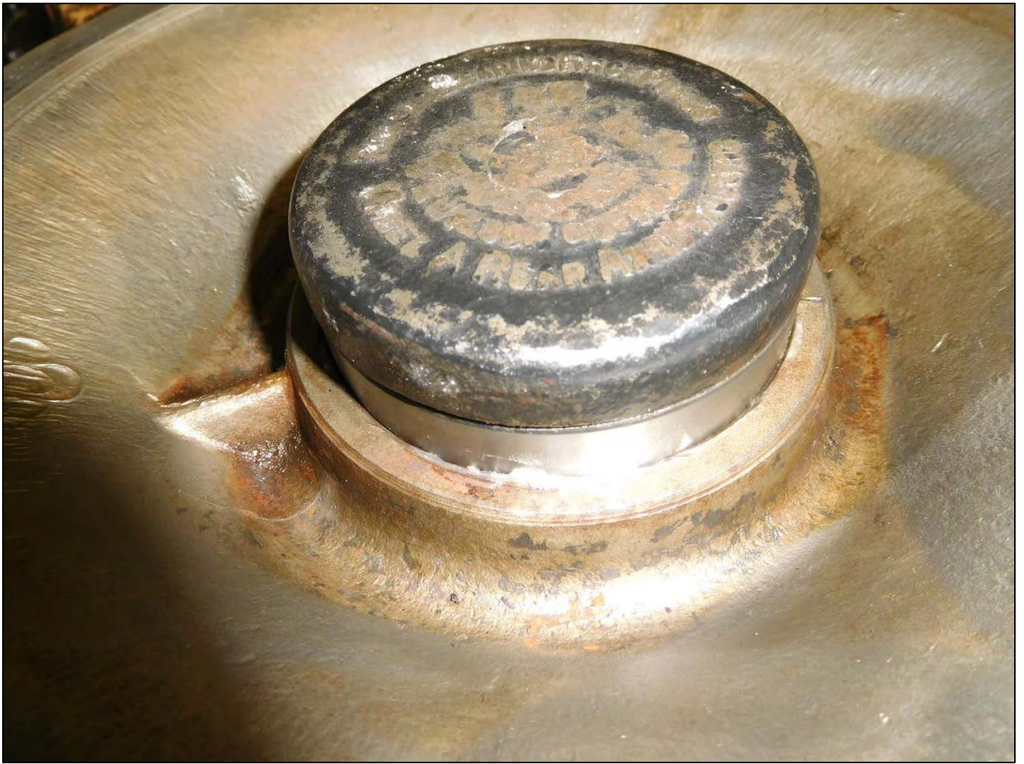
This photo shows a K. R. Wilson tool being used to press the race into place in the axle housing.
