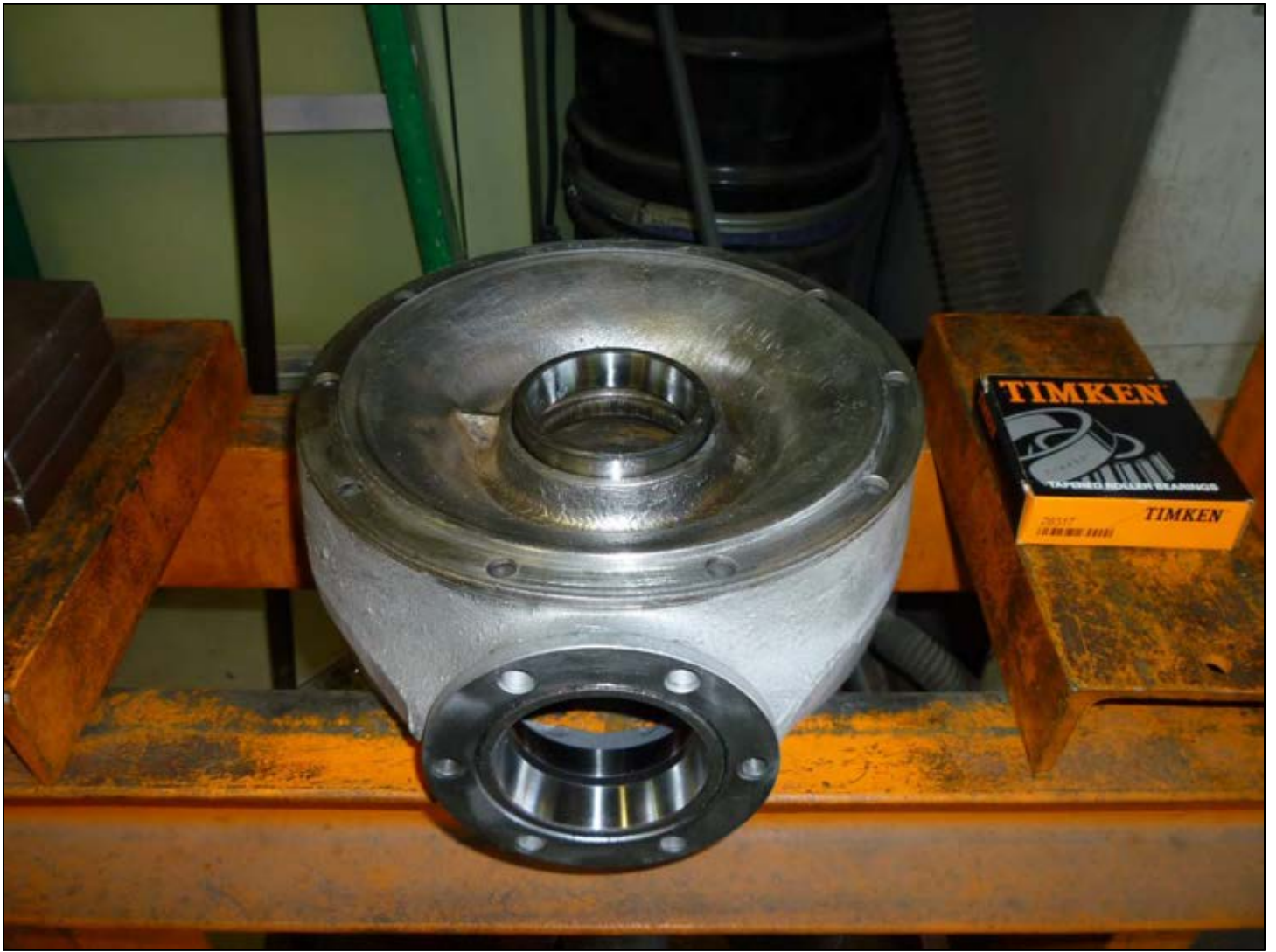
A new axle housing race is set into place.
