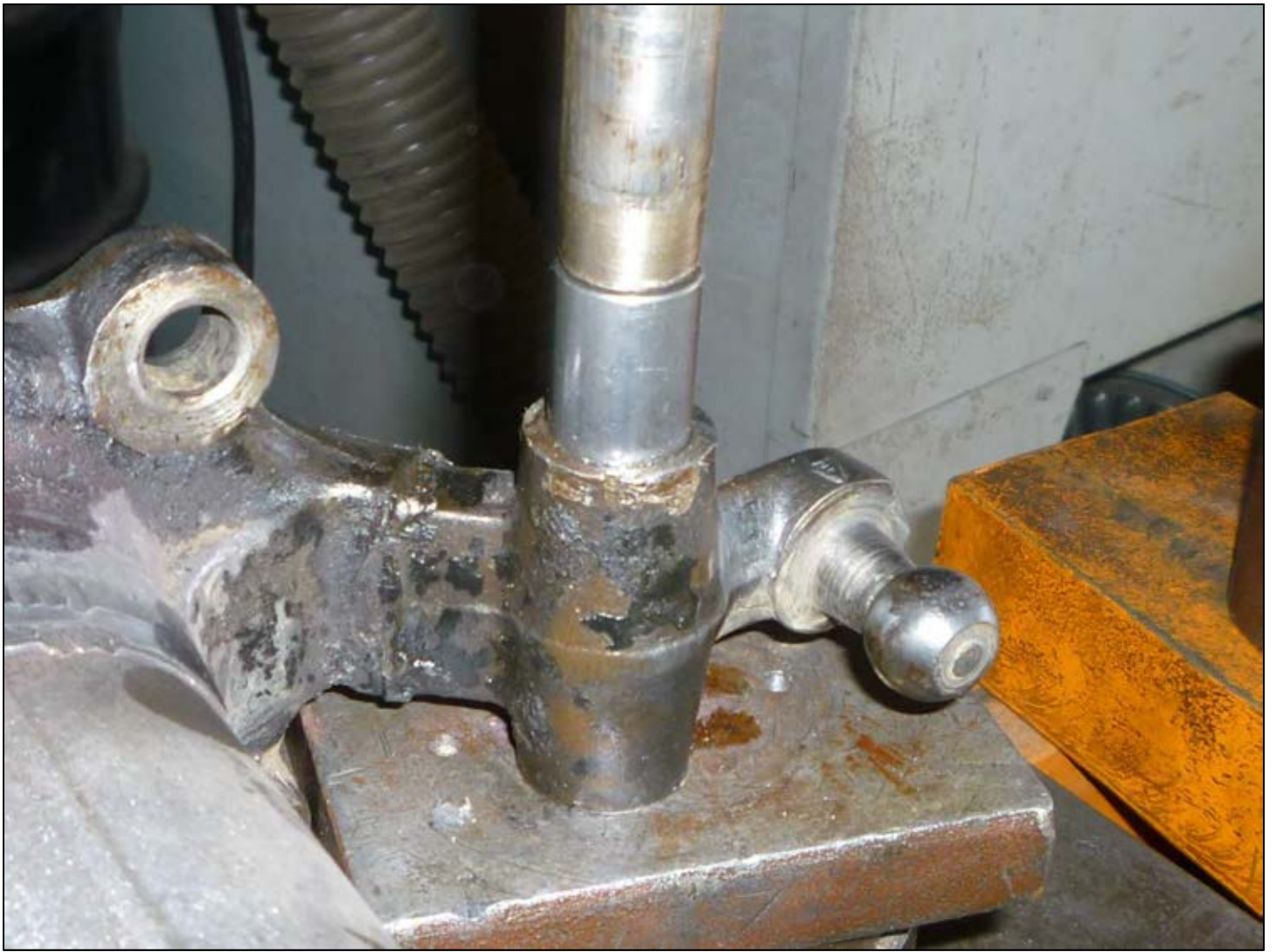
A new shackle bushing is pressed into place.
