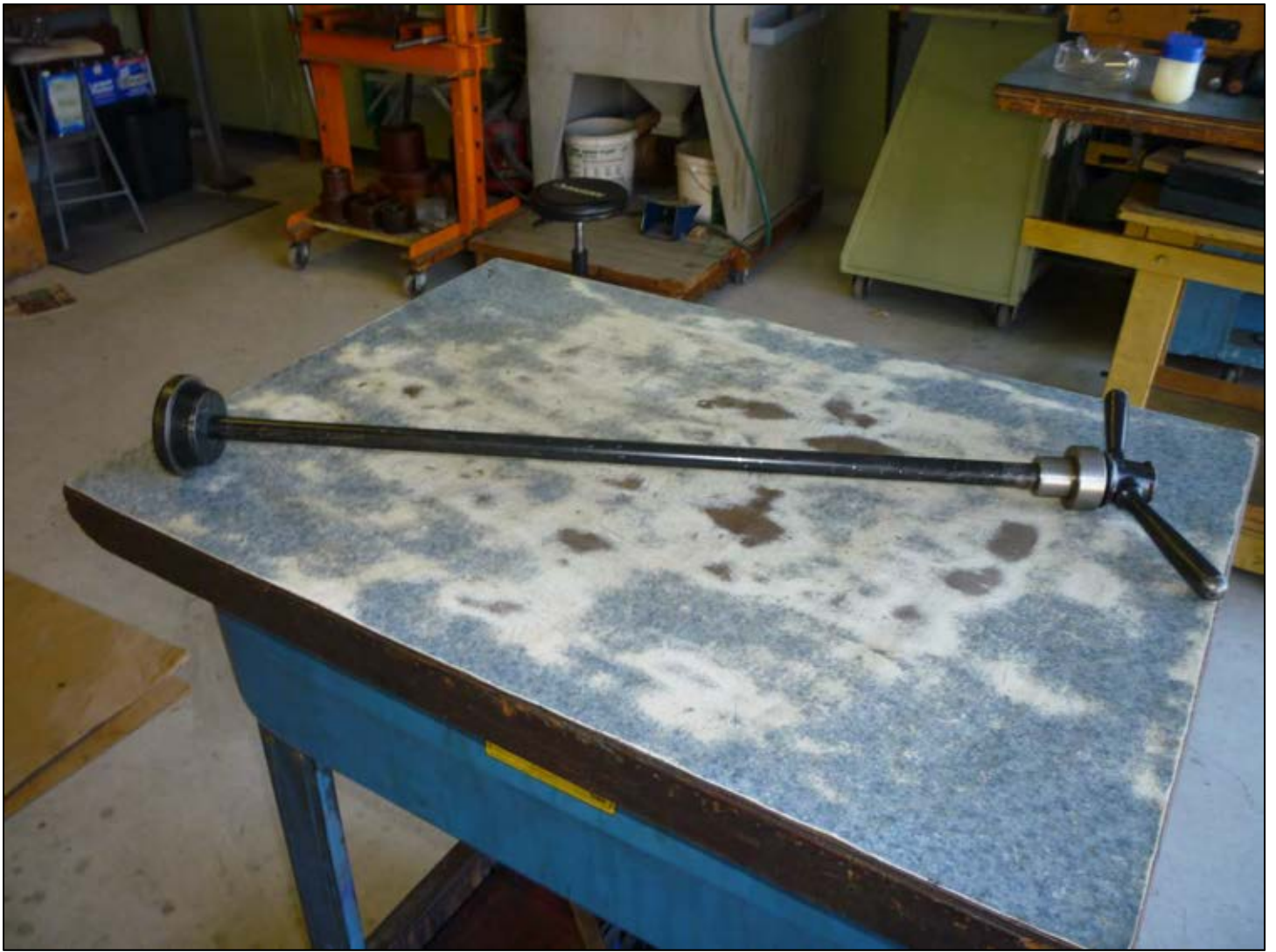
A K.R. Wilson axle housing race presser-inner tool is shown here. It will be used to install the race.
