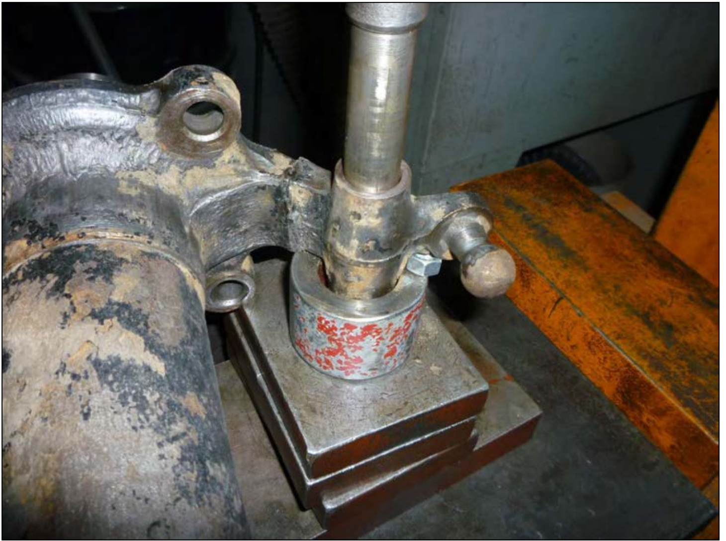
The old shackle bushing is being pressed out with a pusher-outer tool.
