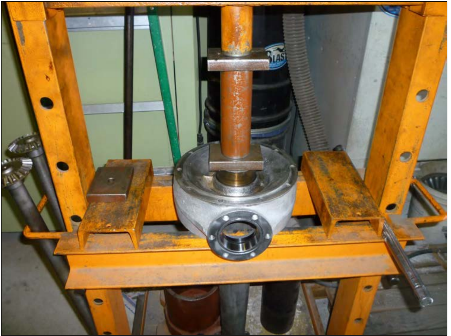
An old banjo race is used to press the new axle housing race into place.
