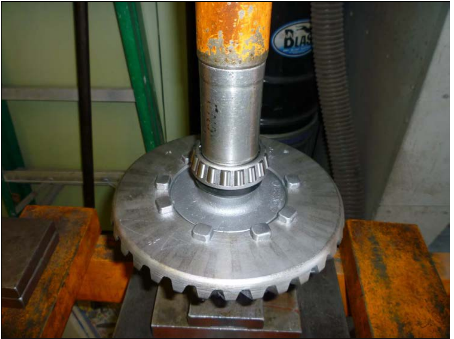
A new bearing is pressed onto the ring gear half of the carrier.
