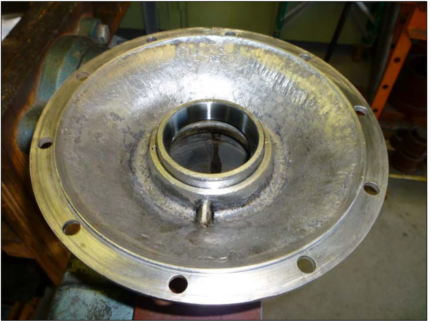
A new race had been set into place and is ready to be pressed in.
