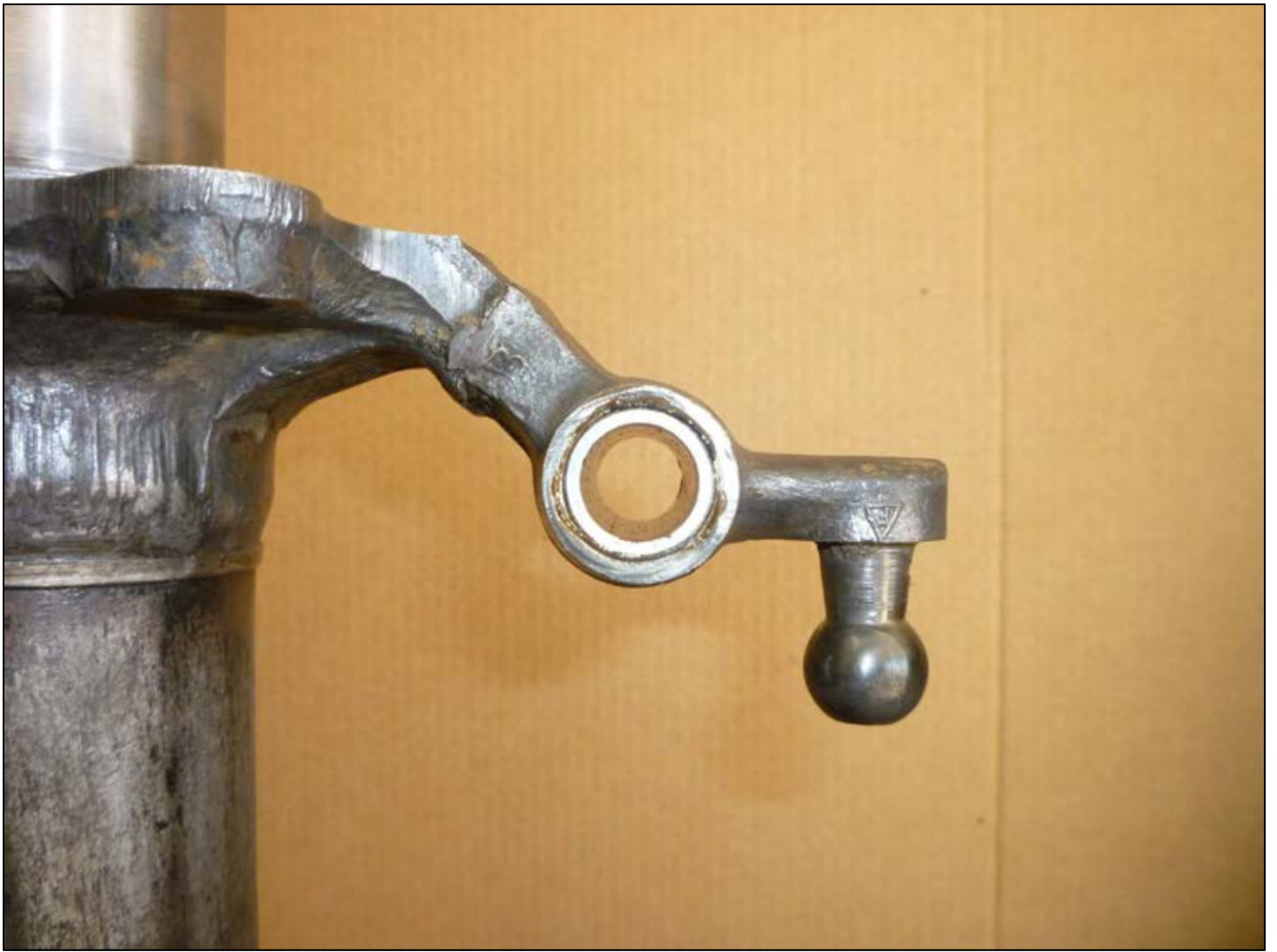
A new shackle bushing has been installed.
