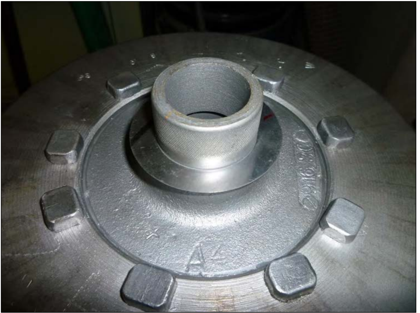
The ring gear carrier half also requires a .005" shim. It is shown in place.
