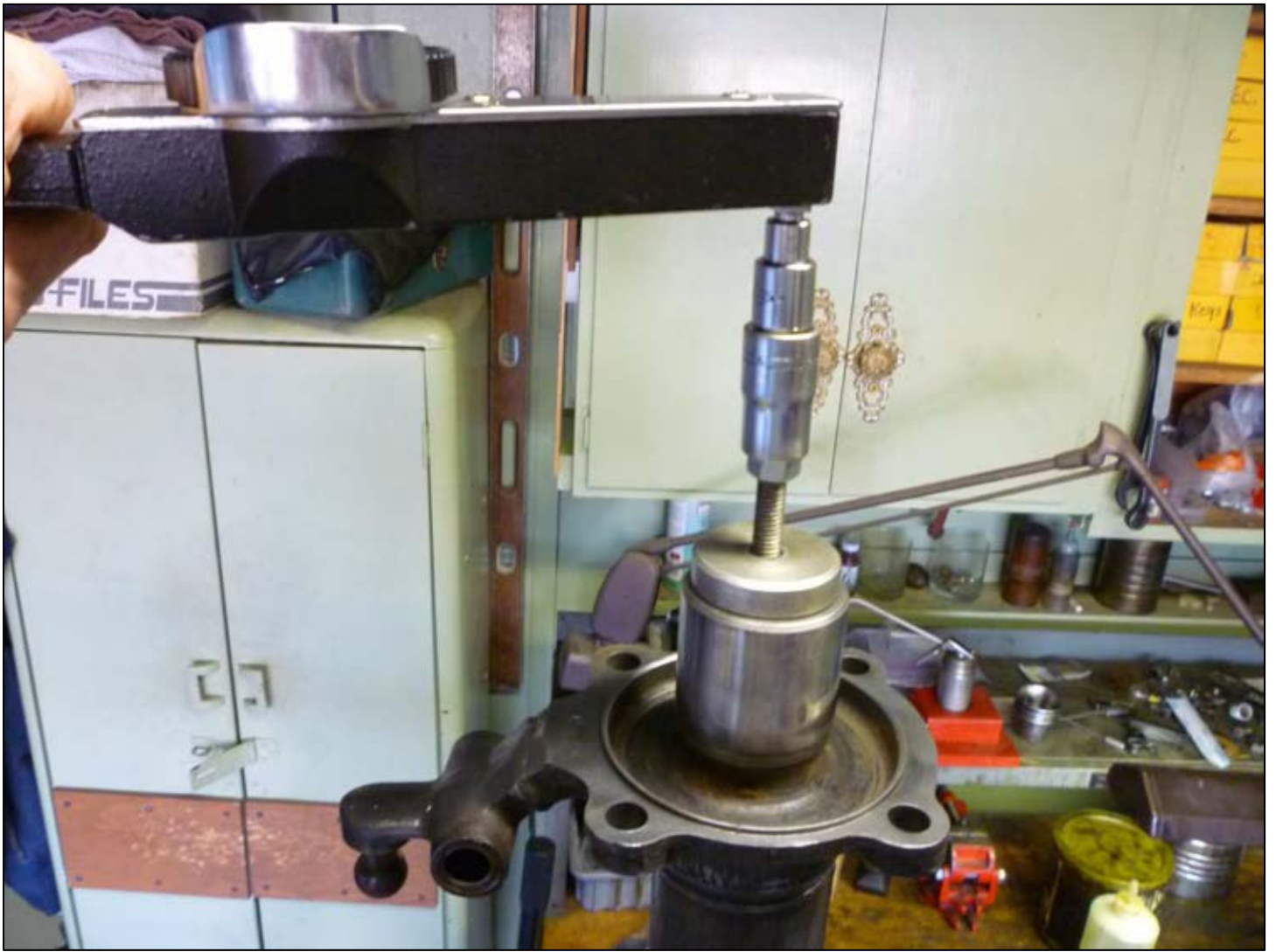
Shown here is the inch pound torque wrench being used to measure the carrier bearing torque value.
