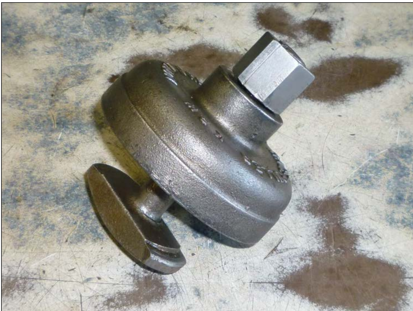
The tool shown is a K.R. Wilson axle housing race removal tool.
