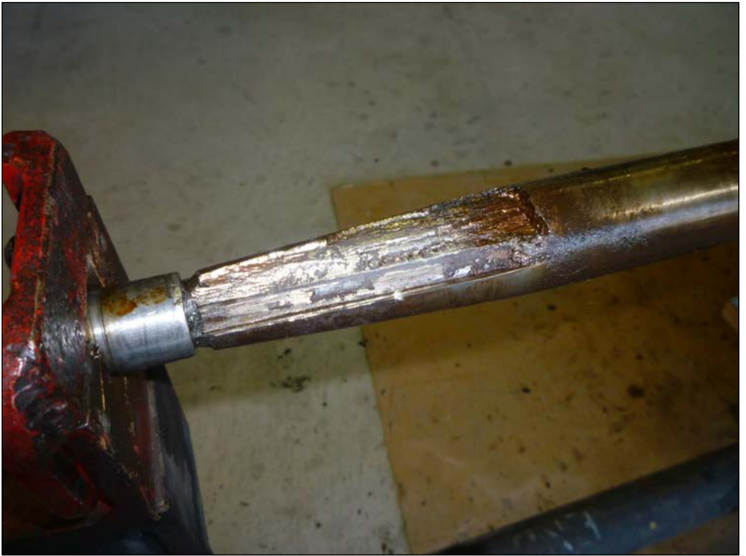
A closer look at the damaged right axle shaft:
