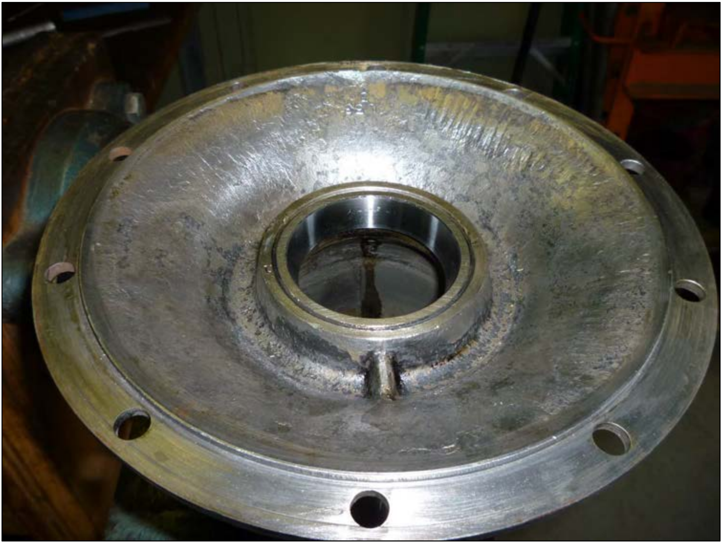
A new race is shown installed.
