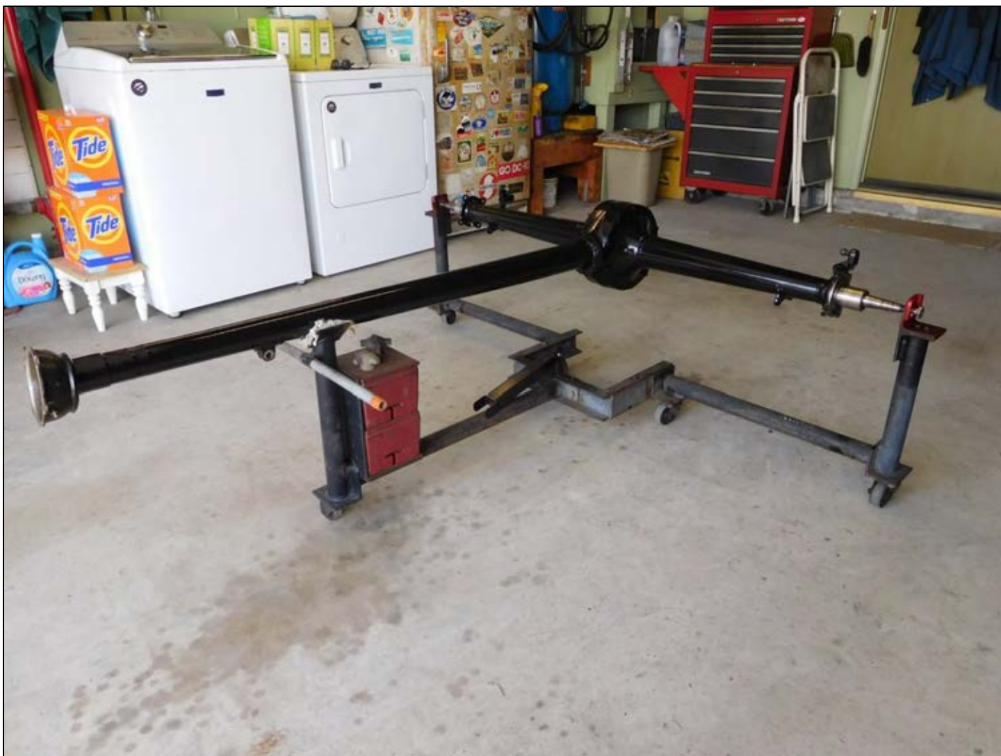
The finished 1932 rear axle assembly, ready for installation back in the car:
