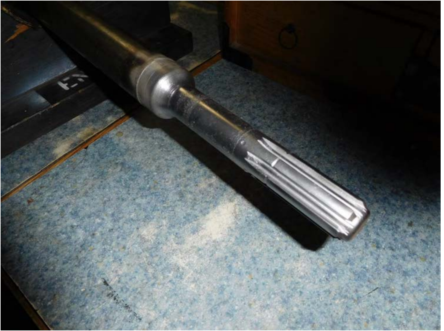
Shown here is the front end of the drive shaft. A hollow tube is installed over the smaller diameter drive shaft and welded into place. The splined end will connect to a U-joint the same as a Model A.
