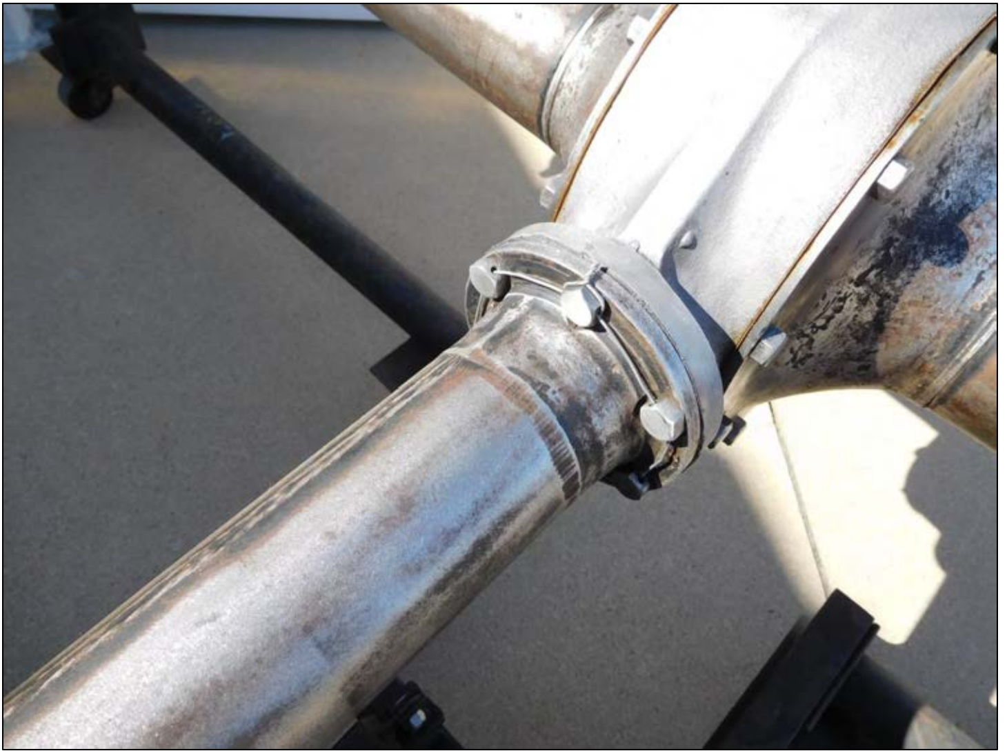
The torque tube bolts have been securely tightened and safety wired in a hallmark perfect circle.
