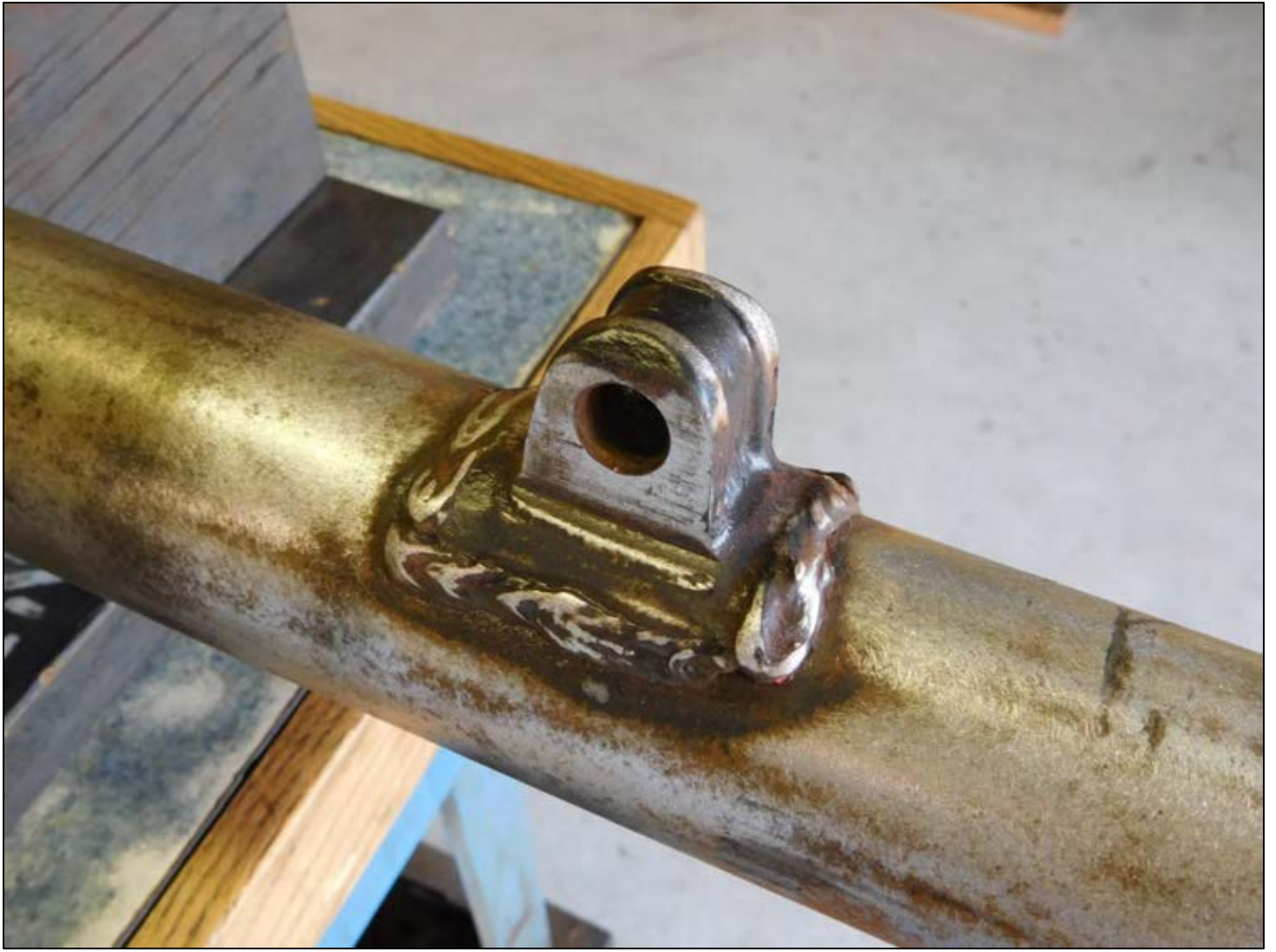
A close up of the bracket that the two radius rods bolt to.
