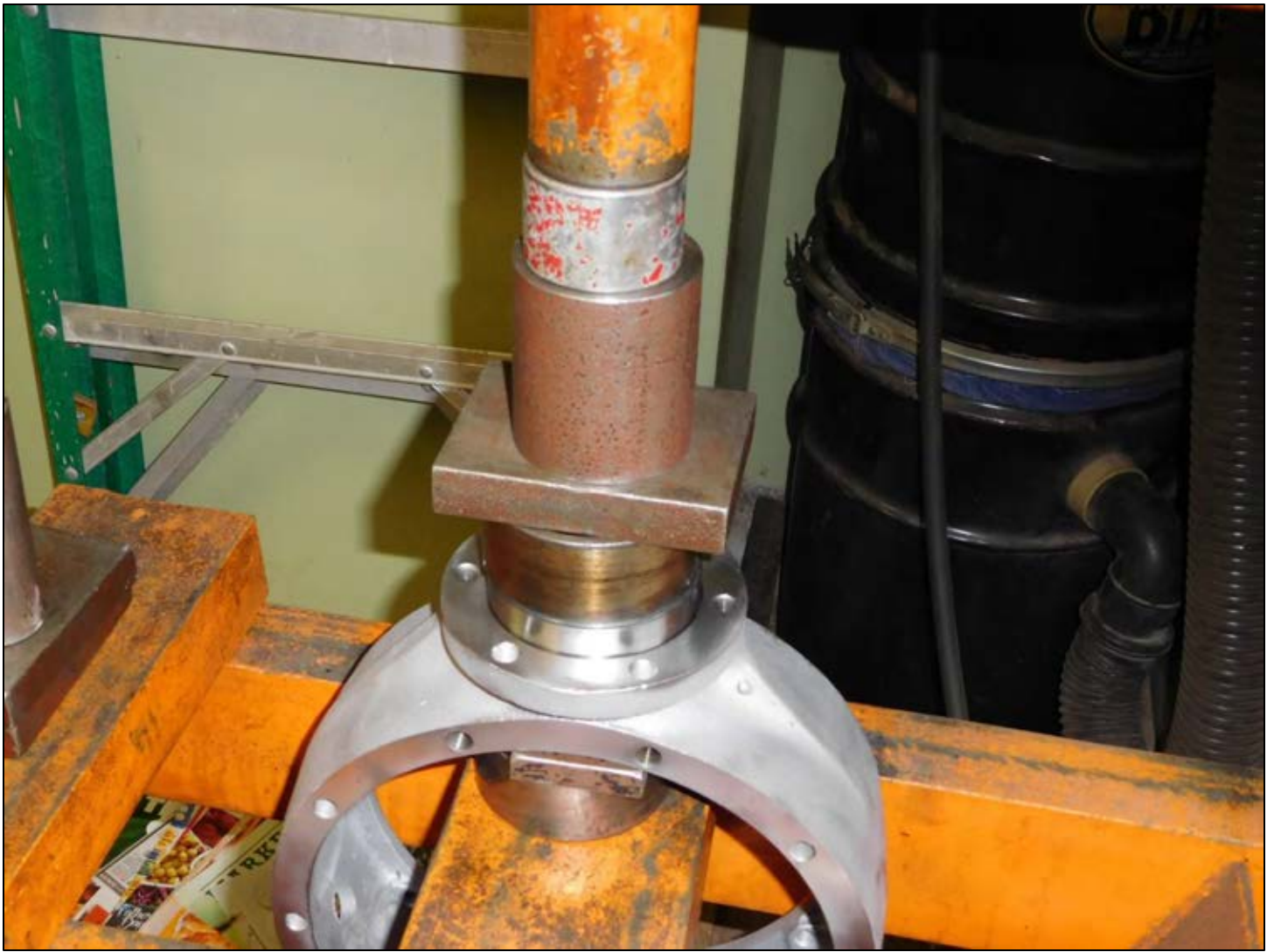
Shown here is the banjo after it was de-greased and bead blasted. A new pinion gear bearing double race is being pressed into place.
