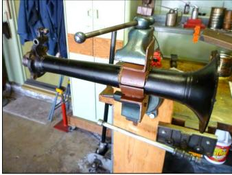
The vice can be swiveled to place an axle housing in a horizontal position for inspection and further cleaning of the inside.
