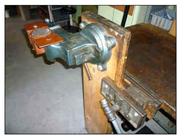
In order to evenly clamp the laminated vertical board in the wood vice a piece of the laminated board is inserted into the vice on the right side.
