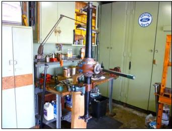
A rear axle assembly with a Mitchell stub shaft is seen clamped in the vertical jig.
