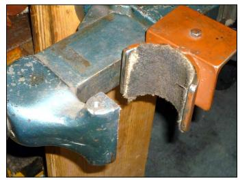
The two angle iron sections are screwed to the top of the vice where holes have been drilled.
