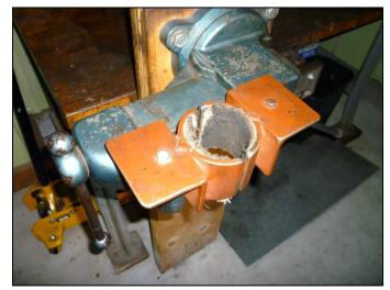
The laminated board has a steel plate screwed to the bottom to prevent the bottom from being worn away each time the jig is removed and dragged from the wood bench vice.
