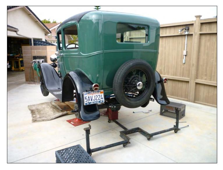
A Model A Ford has been positioned on the tall jack stands. The rear wheels have been removed. The rolling cradle has been positioned beneath the rear of the car and the spring spreader has been installed. The rear axle assembly is ready to come out. Once the cradle is fully under the car a floor jack will be placed under the banjo.
