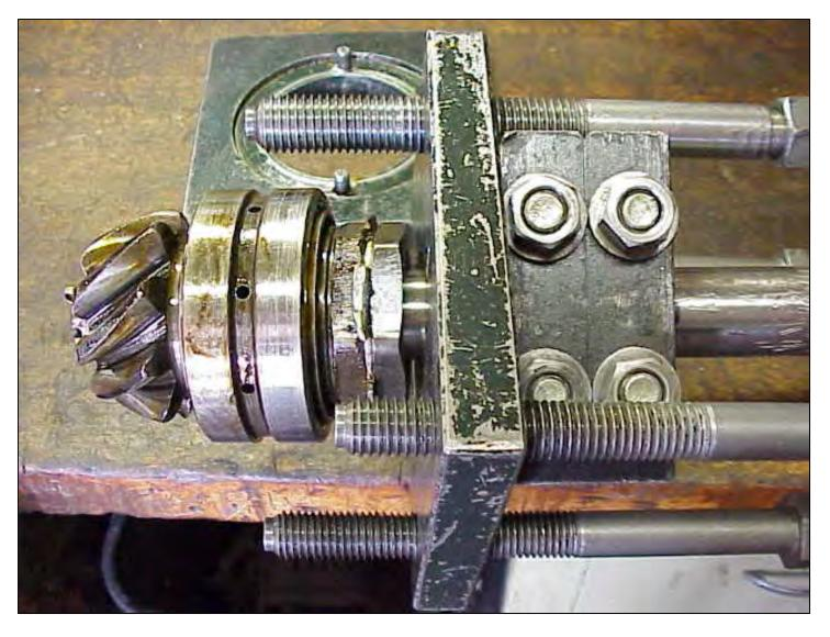
The pinion gear assembly has been pulled from the banjo without disturbing the preload on the two pinion bearings.
