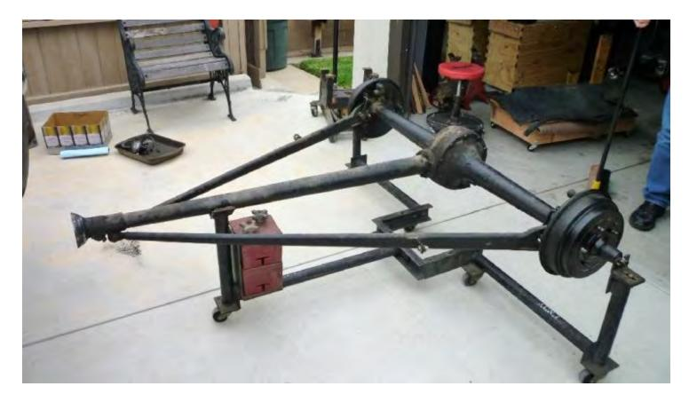
The rear axle assembly has been removed from the car. The torque tube is ready to come off. The rear spring is still attached to the frame of the car with the spring spreader still installed.
