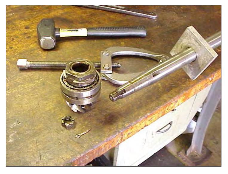
The pinion assembly has been removed from the drive shaft without disturbing the bearing pre-load.
