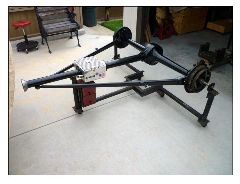
The Mitchell overdrive has been installed onto the rear axle assembly and it is ready to go back into the car. A floor jack can be seen behind the rear axle assembly. It has a fixture on it that fits directly under the banjo and captures both axle housings. The U-shape structure on the rolling cradle allows the jack to be positioned directly under the banjo.
