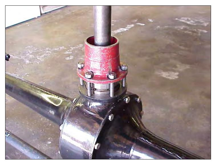
The pinion gear assembly attached to the Mitchell stub shaft is being reinstalled into the banjo using a puller-in tool. By tightening the nuts on the threaded studs evenly it will seat the pinion assembly into the banjo.
