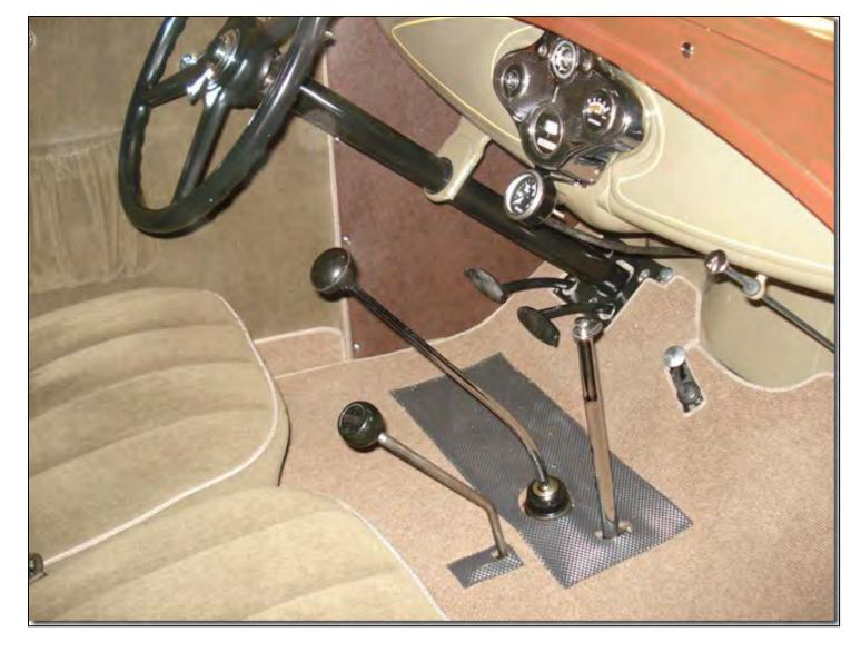
A template was used to locate the slot in the floor board for the overdrive shift lever to protrude through. The shifting mechanism can be adjusted to provide desired fore and aft positioning of the shift lever.
