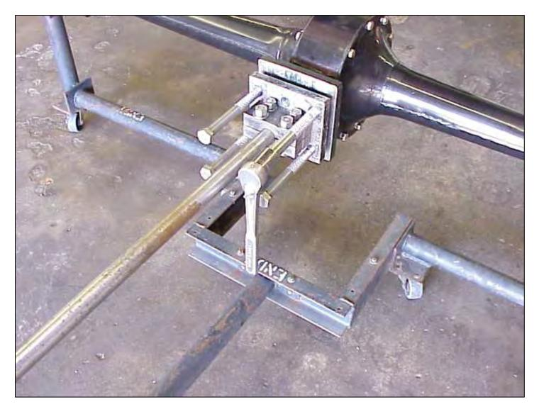
The torque tube has been removed and discarded. The pinion assembly and drive shaft are being removed from the banjo with the pinion gear assembly puller.
