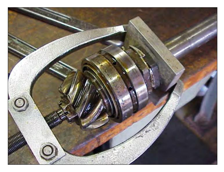
The pinion assembly is removed from the drive shaft with a puller tool without disturbing the pre-load on the pinion bearings. The puller is tightened against the block of steel that has a hole in it to allow it to slide over the drive shaft ad up against the pinion assembly. The end of the puller is hit with a hammer to dislodge the pinion assembly from the tapered shaft.
