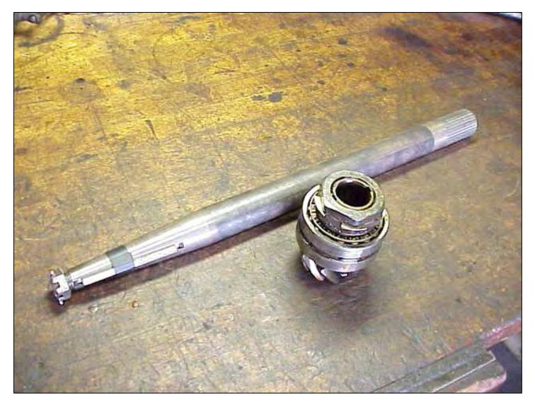
The Mitchell stub shaft is ready to be installed into the removed pinion gear assembly. The nut will be torqued to 100 ft. lbs.
