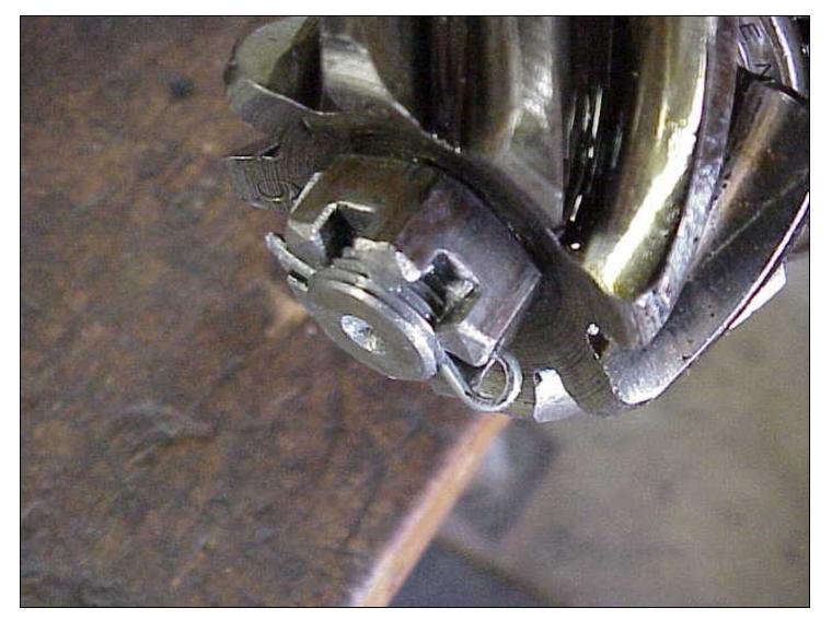
The cotter pin will be removed from the end of the drive shaft and the nut loosened and backed off about 1/8".
