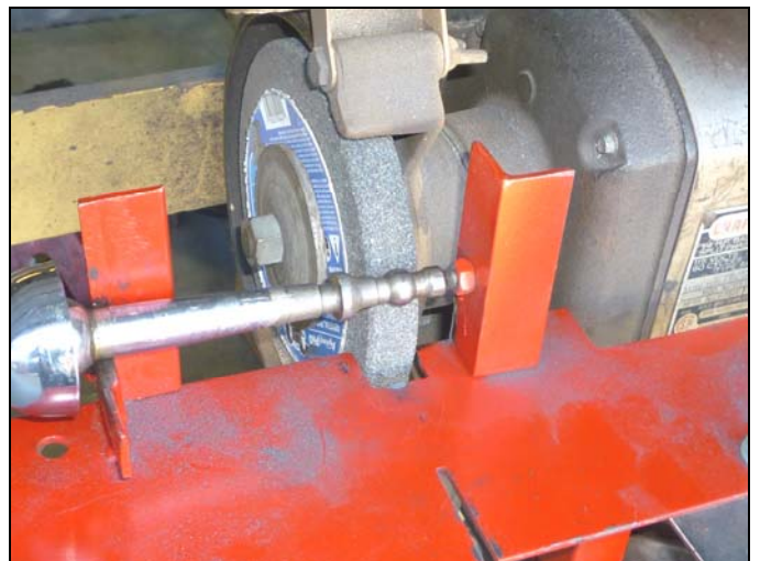
A bench grinder jig for grinding down the welded ball on the end of shifting levers:
