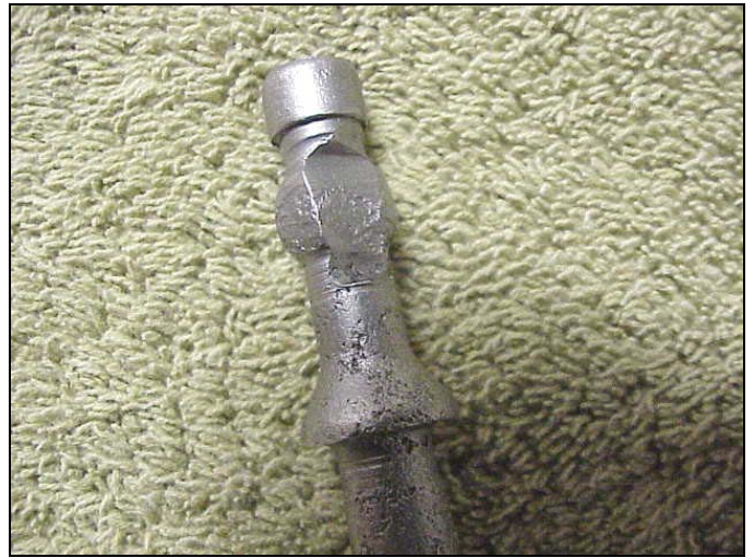
The ball on the end of the shift lever has to be welded up and ground down to restore the original 1/2" diameter:
