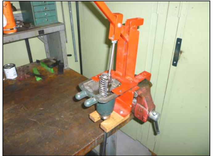
Quick and easy killer spring removal and installation tool:
