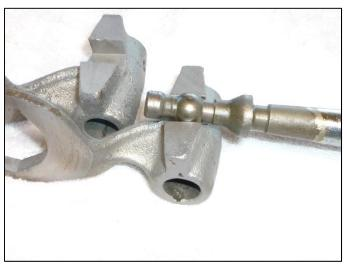
The slots in the two reproduction forks are not wide enough to allow the ball on the end of the shifter to travel inside the slots without becoming jammed.
