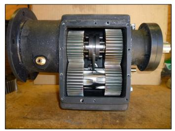
A Ryan overdrive still new in the box was discovered at a swap meet. The four gears never come out of mesh. The two on the right are replaced to change from a 23% to a 33% This one is a 23%.
