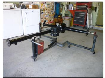
The new Ryan 23% overdrive installed on a newly overhauled rear axle assembly:
