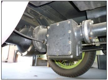
The 23% Ryan overdrive installed in my Victoria in 1994 has over 50,000 miles on it. The back of the dropped floor pan was cut away to provide clearance for the overdrive.
