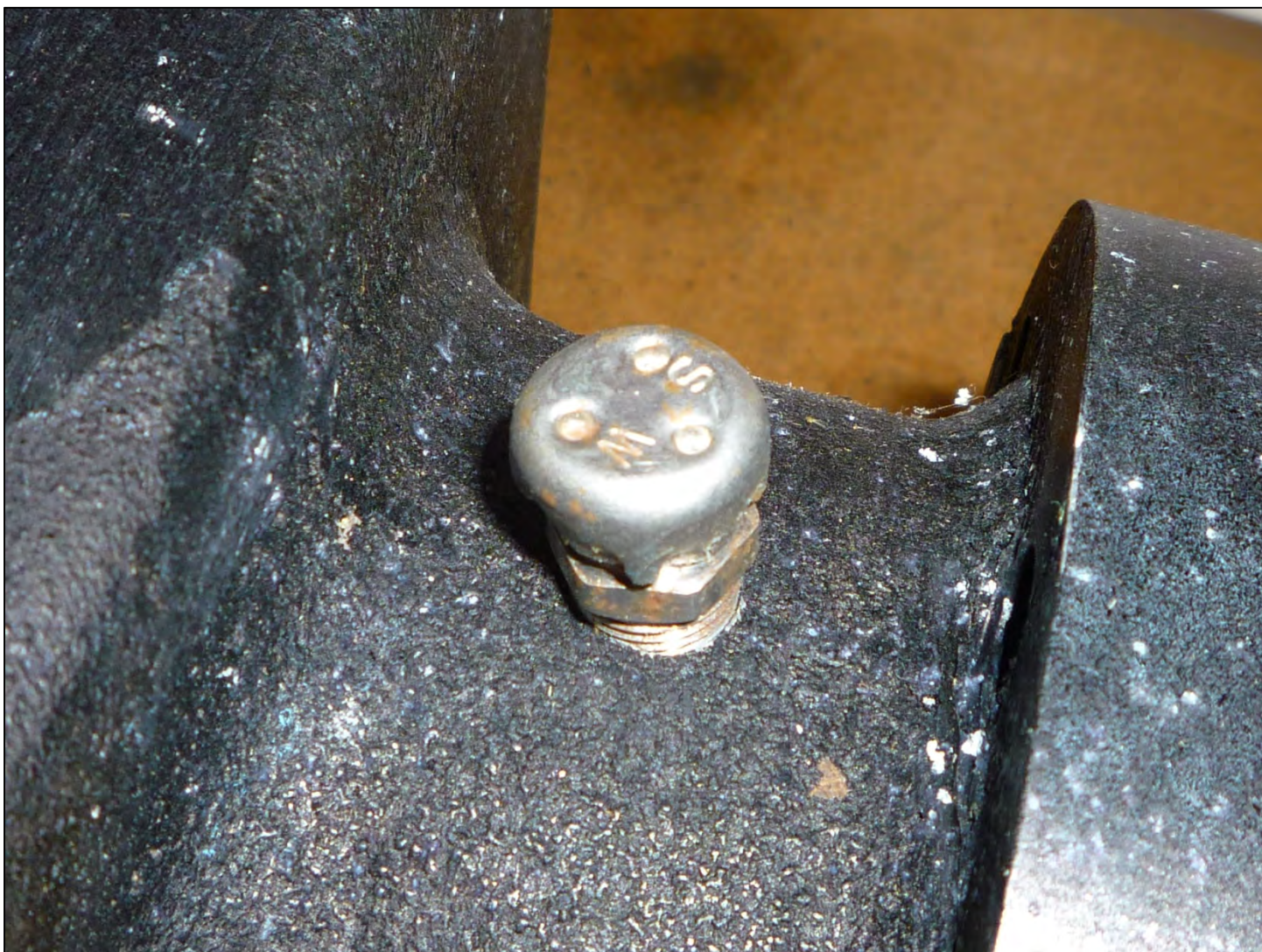
A close up view of the vent valve on top of the Ryan gear box:
